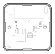
The "LINK" LED on the Ethernet connector indicates both status of the Ethernet Link level and if communication is ongoing.
