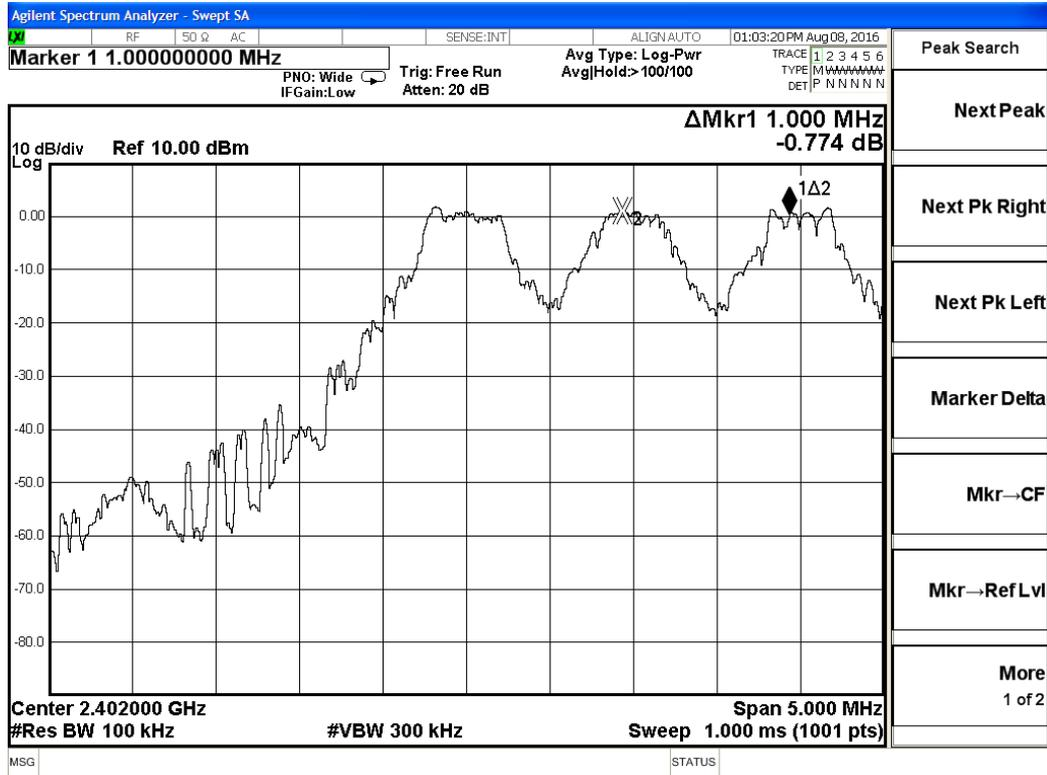
**Test Plot Of Frequency Separation (2Mbps)**
