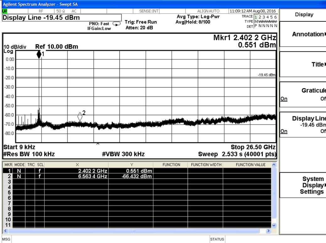
**9KHz-26.5GHz Middle Channel(8-DPSK)**
