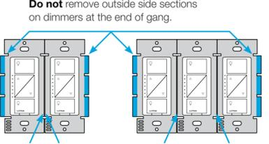
Each dimmer has inside side sections removed. Dimmer at middle has all side sections removed.
