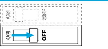
**WARNING: SHOCK HAZARD.** May result in serious injury or death. Turn off power at circuit breaker or fuse before installing.
