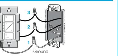
1 Connect the bare copper (or green) "ground" wire from the wallbox to the green wire on the dimmer using a wire connector.
