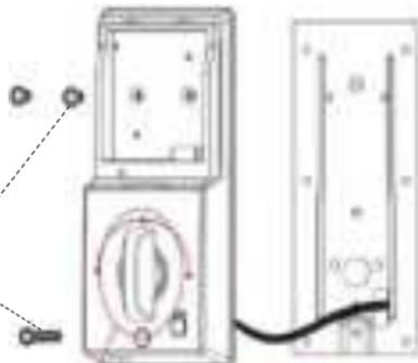
The screws must be pushed to the vertical stop.
