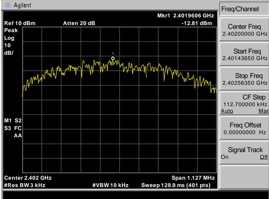
Test Model Power Spectral Density
