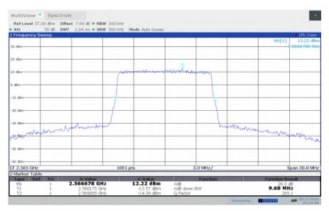
LTE band 7, 10MHz Bandwidth, HIGH, 64QAM (-26dBc BW)
