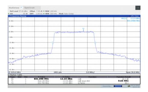
LTE band 5, 10MHz Bandwidth, MID, QPSK (-26dBc BW)
