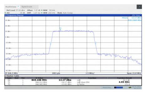
LTE band 5, 5MHz Bandwidth, HIGH, 64QAM (-26dBc BW)
