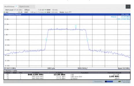
LTE band 5, 3MHz Bandwidth, HIGH, 64QAM (-26dBc BW)
