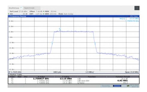
LTE band 4, 5MHz Bandwidth, MID, 64QAM (-26dBc BW)
