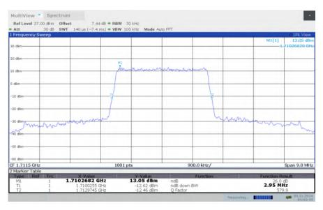
LTE band 4, 3MHz Bandwidth, LOW, 16QAM (-26dBc BW)
