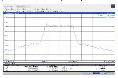
LTE band 5, 1.4MHz Bandwidth, LOW, 64QAM (-26dBc BW)
