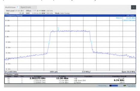
LTE band 7, 10MHz Bandwidth, LOW, 64QAM (-26dBc BW)
