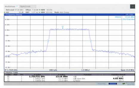
LTE band 4, 5MHz Bandwidth, MID, 16QAM (-26dBc BW)
