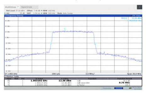
LTE band 2, 10MHz Bandwidth, HIGH, 64QAM (-26dBc BW)
