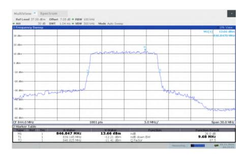
LTE band 5, 10MHz Bandwidth, HIGH, 16QAM (-26dBc BW)
