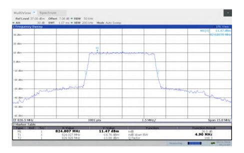
LTE band 5, 5MHz Bandwidth, MID, QPSK (-26dBc BW)
