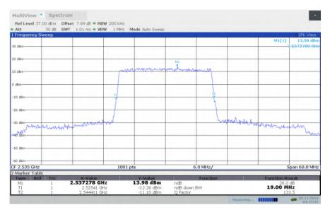
LTE band 7, 20MHz Bandwidth, MID, 16QAM (-26dBc BW)
