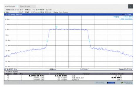
LTE band 2, 5MHz Bandwidth, HIGH, 64QAM (-26dBc BW)
