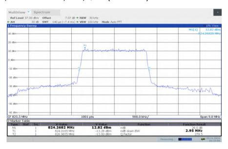
LTE band 5, 3MHz Bandwidth, LOW, 16QAM (-26dBc BW)
