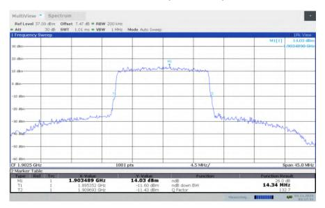
LTE band 2, 15MHz Bandwidth, HIGH, 64QAM (-26dBc BW)
