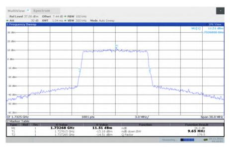
LTE band 4, 10MHz Bandwidth, HIGH, QPSK (-26dBc BW)
