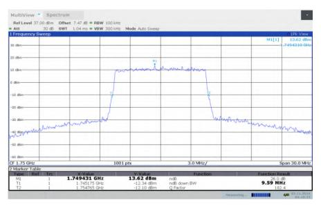
LTE band 4, 10MHz Bandwidth, HIGH, 64QAM (-26dBc BW)
