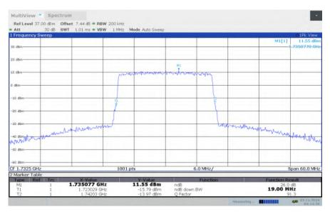
LTE band 4, 20MHz Bandwidth, HIGH, QPSK (-26dBc BW)
