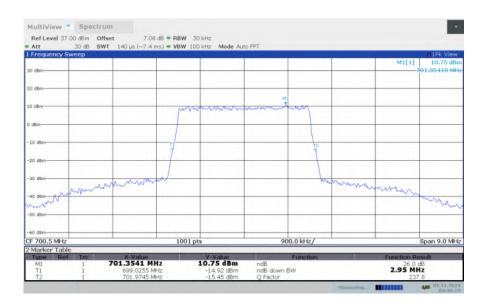
LTE band 12, 3MHz Bandwidth, MID, QPSK (-26dBc BW)
