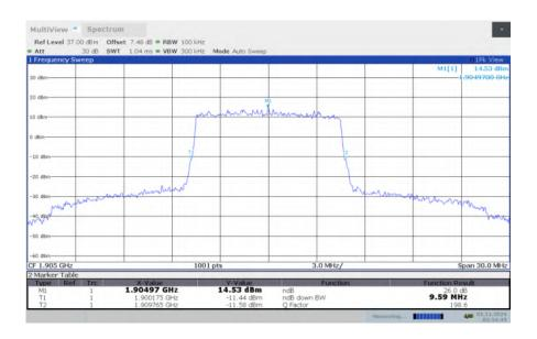
LTE band 2, 10MHz Bandwidth, HIGH, 16QAM (-26dBc BW)
