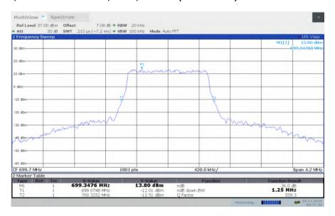
LTE band 12, 1.4MHz Bandwidth, LOW, 64QAM (-26dBc BW)
