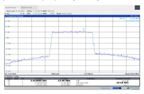
LTE band 7, 20MHz Bandwidth, LOW, 64QAM (-26dBc BW)
