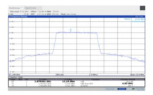
LTE band 2, 5MHz Bandwidth, MID, 64QAM (-26dBc BW)
