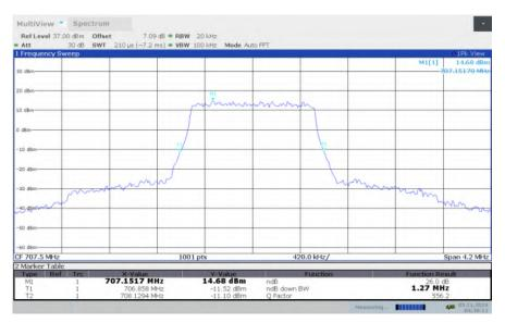
LTE band 12, 1.4MHz Bandwidth, MID, 16QAM (-26dBc BW)
