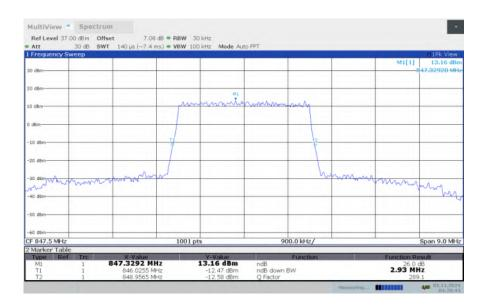
LTE band 5, 3MHz Bandwidth, HIGH, 16QAM (-26dBc BW)
