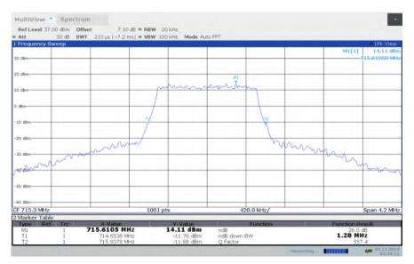
LTE band 12, 1.4MHz Bandwidth, HIGH, 64QAM (-26dBc BW)
