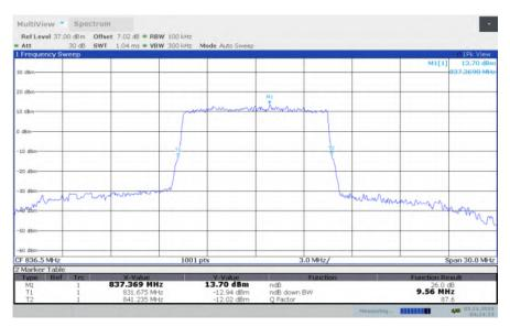
LTE band 5, 10MHz Bandwidth, MID, 16QAM (-26dBc BW)
