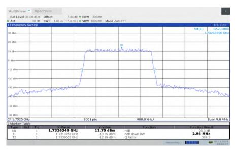
LTE band 4, 3MHz Bandwidth, MID, 16QAM (-26dBc BW)
