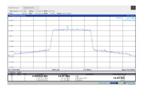
LTE band 7, 15MHz Bandwidth, MID, 64QAM (-26dBc BW)
