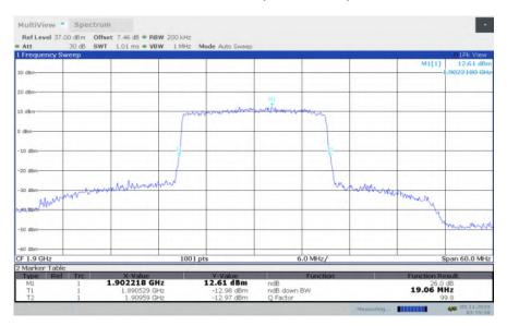
LTE band 2, 20MHz Bandwidth, HIGH, 64QAM (-26dBc BW)
