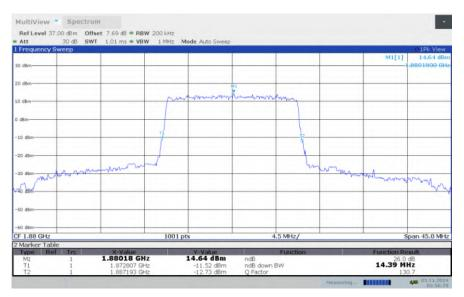
LTE band 2, 15MHz Bandwidth, MID, 16QAM (-26dBc BW)
