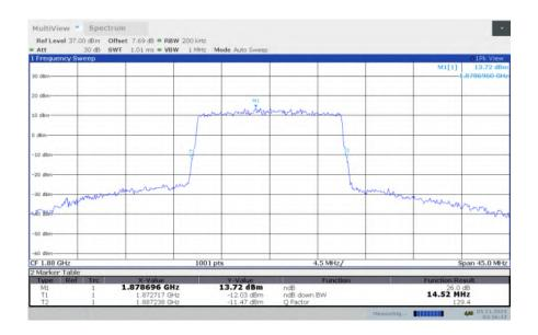
LTE band 2, 15MHz Bandwidth, MID, 64QAM (-26dBc BW)
