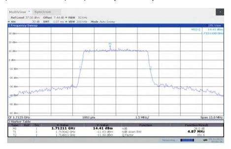
LTE band 4, 5MHz Bandwidth, LOW, 64QAM (-26dBc BW)
