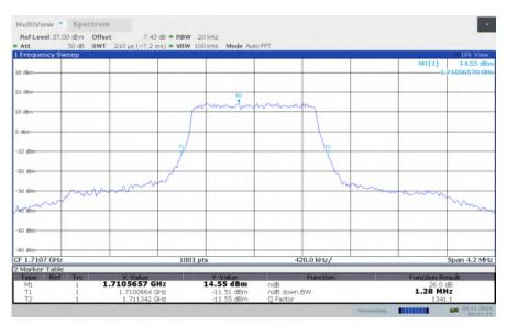
LTE band 4, 1.4MHz Bandwidth, LOW, 16QAM (-26dBc BW)
