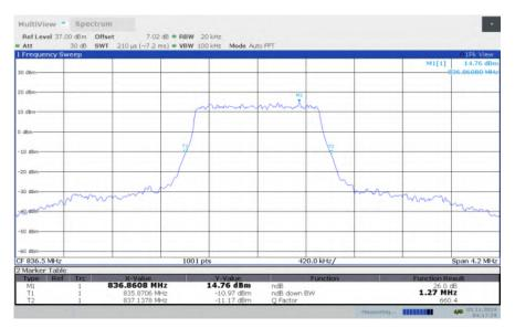
LTE band 5, 1.4MHz Bandwidth, MID, 16QAM (-26dBc BW)
