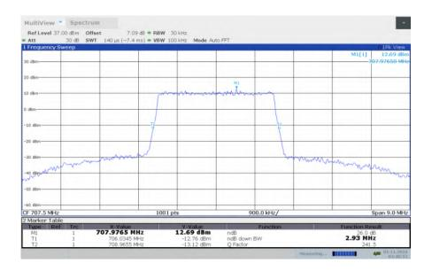
LTE band 12, 3MHz Bandwidth, MID, 64QAM (-26dBc BW)
