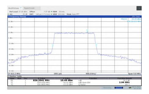
LTE band 5, 3MHz Bandwidth, MID, QPSK (-26dBc BW)
