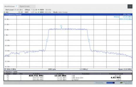
LTE band 5, 5MHz Bandwidth, MID, 16QAM (-26dBc BW)
