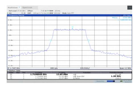
LTE band 4, 1.4MHz Bandwidth, MID, QPSK (-26dBc BW)
