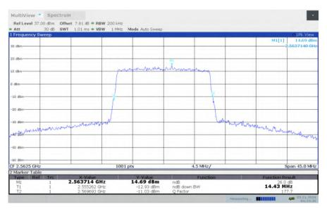
LTE band 7, 15MHz Bandwidth, HIGH, 64QAM (-26dBc BW)
