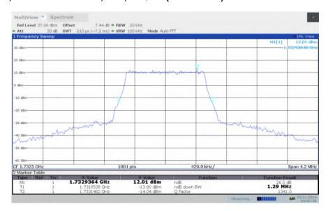
LTE band 4, 1.4MHz Bandwidth, HIGH, QPSK (-26dBc BW)
