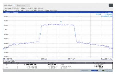
LTE band 2, 10MHz Bandwidth, MID, 16QAM (-26dBc BW)
