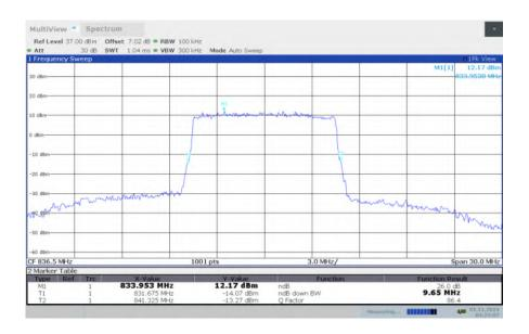
LTE band 5, 10MHz Bandwidth, MID, 64QAM (-26dBc BW)
