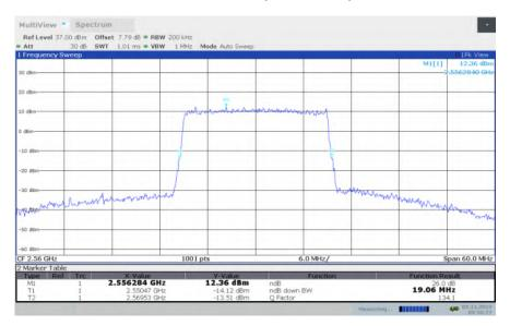
LTE band 7, 20MHz Bandwidth, HIGH, 64QAM (-26dBc BW)
