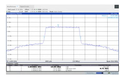
LTE band 2, 10MHz Bandwidth, MID, QPSK (-26dBc BW)
