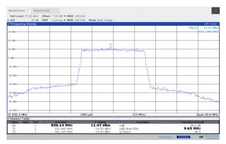
LTE band 5, 10MHz Bandwidth, HIGH, QPSK (-26dBc BW)
