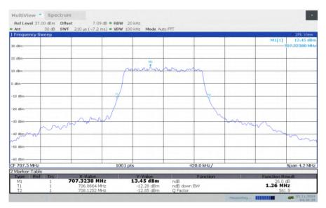
LTE band 12, 1.4MHz Bandwidth, HIGH, QPSK (-26dBc BW)
