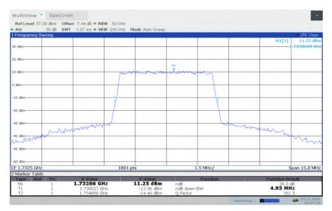
LTE band 4, 5MHz Bandwidth, HIGH, QPSK (-26dBc BW)
