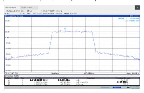
LTE band 4, 3MHz Bandwidth, LOW, 64QAM (-26dBc BW)
