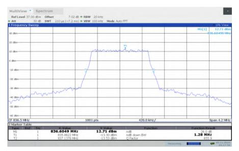
LTE band 5, 1.4MHz Bandwidth, HIGH, QPSK (-26dBc BW)
