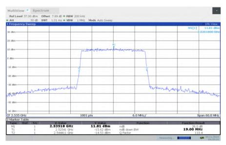
LTE band 7, 20MHz Bandwidth, HIGH, QPSK (-26dBc BW)
