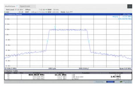
LTE band 5, 3MHz Bandwidth, HIGH, QPSK (-26dBc BW)
