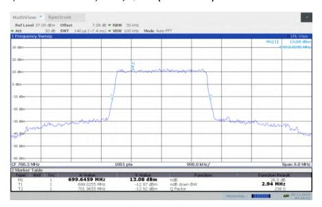
LTE band 12, 3MHz Bandwidth, LOW, 16QAM (-26dBc BW)
