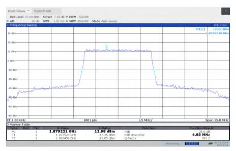
LTE band 2, 5MHz Bandwidth, MID, 16QAM (-26dBc BW)
