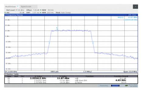
LTE band 7, 5MHz Bandwidth, HIGH, QPSK (-26dBc BW)
