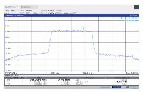
LTE band 12, 3MHz Bandwidth, MID, 16QAM (-26dBc BW)
