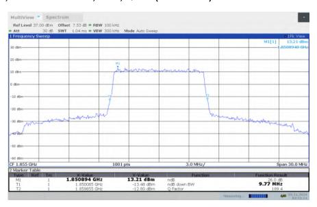
LTE band 2, 10MHz Bandwidth, LOW, 16QAM (-26dBc BW)
