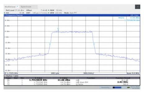
LTE band 4, 3MHz Bandwidth, HIGH, QPSK (-26dBc BW)
