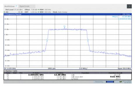
LTE band 7, 10MHz Bandwidth, HIGH, QPSK (-26dBc BW)
