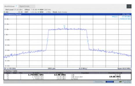
LTE band 4, 20MHz Bandwidth, HIGH, 64QAM (-26dBc BW)
