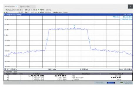
LTE band 4, 5MHz Bandwidth, LOW, 16QAM (-26dBc BW)
