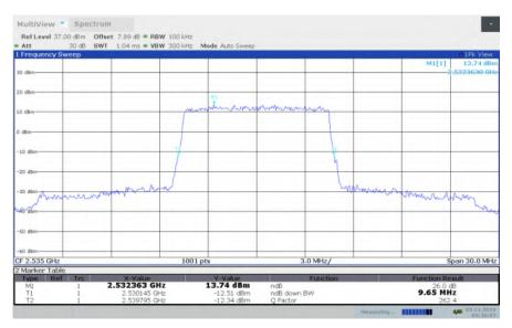
LTE band 7, 10MHz Bandwidth, MID, 16QAM (-26dBc BW)
