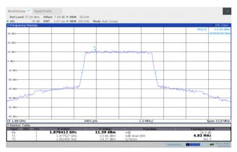
LTE band 2, 5MHz Bandwidth, HIGH, QPSK (-26dBc BW)
