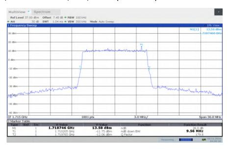
LTE band 4, 10MHz Bandwidth, LOW, 64QAM (-26dBc BW)
