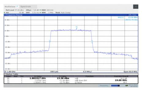
LTE band 2, 20MHz Bandwidth, MID, 16QAM (-26dBc BW)
