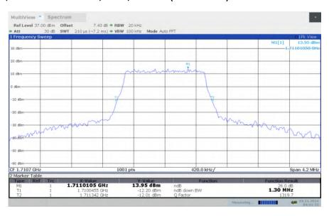
LTE band 4, 1.4MHz Bandwidth, LOW, 64QAM (-26dBc BW)
