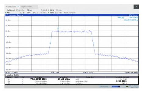
LTE band 12, 3MHz Bandwidth, HIGH, QPSK (-26dBc BW)
