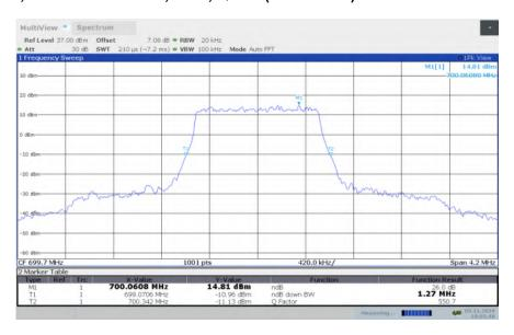
LTE band 12, 1.4MHz Bandwidth, LOW, 16QAM (-26dBc BW)
