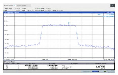
LTE band 5, 3MHz Bandwidth, MID, 16QAM (-26dBc BW)
