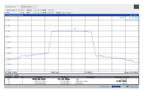
LTE band 5, 5MHz Bandwidth, HIGH, QPSK (-26dBc BW)
