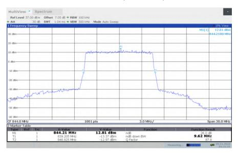
LTE band 5, 10MHz Bandwidth, HIGH, 64QAM (-26dBc BW)
