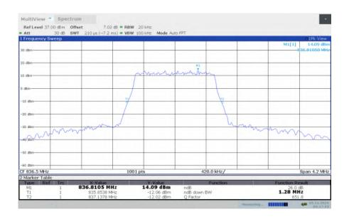
LTE band 5, 1.4MHz Bandwidth, MID, 64QAM (-26dBc BW)
