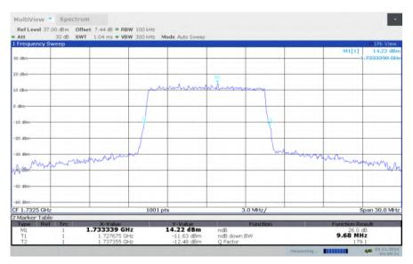
LTE band 4, 10MHz Bandwidth, MID, 16QAM (-26dBc BW)
