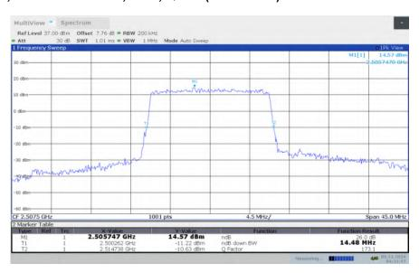
LTE band 7, 15MHz Bandwidth, LOW, 16QAM (-26dBc BW)
