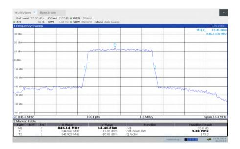
LTE band 5, 5MHz Bandwidth, HIGH, 16QAM (-26dBc BW)
