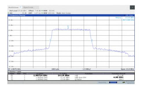
LTE band 2, 5MHz Bandwidth, HIGH, 16QAM (-26dBc BW)
