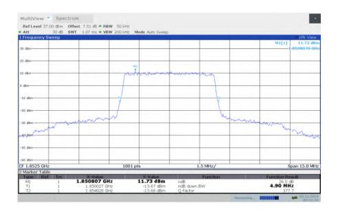
LTE band 2, 5MHz Bandwidth, MID, QPSK (-26dBc BW)
