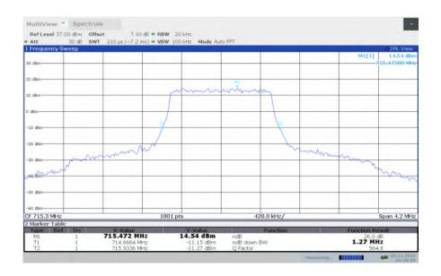
LTE band 12, 1.4MHz Bandwidth, HIGH, 16QAM (-26dBc BW)
