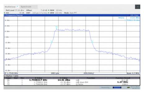
LTE band 4, 1.4MHz Bandwidth, HIGH, 64QAM (-26dBc BW)
