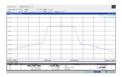
LTE band 5, 1.4MHz Bandwidth, MID, QPSK (-26dBc BW)
