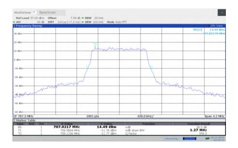
LTE band 12, 1.4MHz Bandwidth, MID, 64QAM (-26dBc BW)
