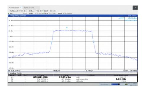
LTE band 5, 5MHz Bandwidth, MID, 64QAM (-26dBc BW)
