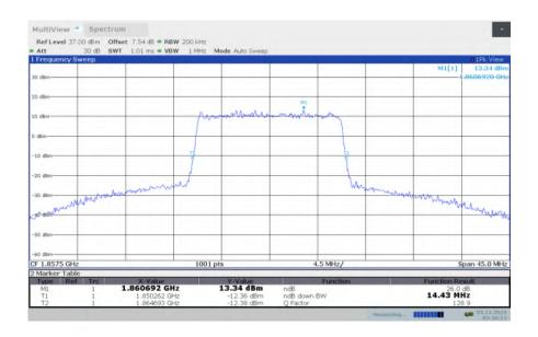
LTE band 2, 15MHz Bandwidth, MID, QPSK (-26dBc BW)
