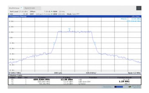
LTE band 12, 1.4MHz Bandwidth, MID, QPSK (-26dBc BW)
