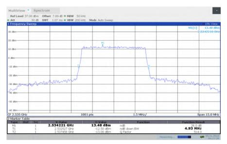
LTE band 7, 5MHz Bandwidth, MID, 16QAM (-26dBc BW)
