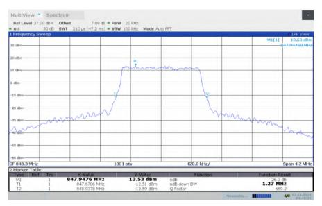
LTE band 5, 1.4MHz Bandwidth, HIGH, 64QAM (-26dBc BW)
