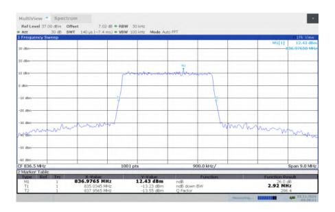
LTE band 5, 3MHz Bandwidth, MID, 64QAM (-26dBc BW)
