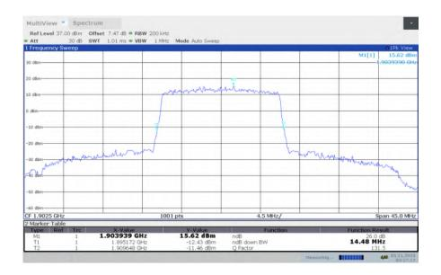
LTE band 2, 15MHz Bandwidth, HIGH, 16QAM (-26dBc BW)
