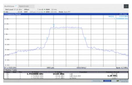
LTE band 4, 1.4MHz Bandwidth, MID, 16QAM (-26dBc BW)
