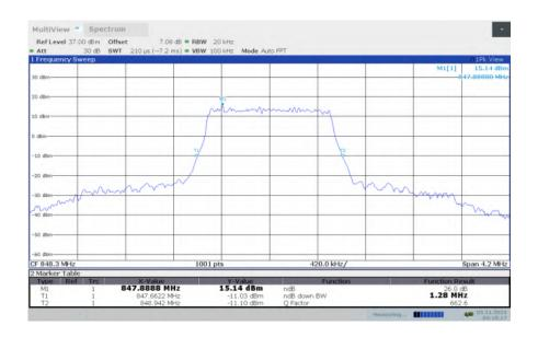
LTE band 5, 1.4MHz Bandwidth, HIGH, 16QAM (-26dBc BW)
