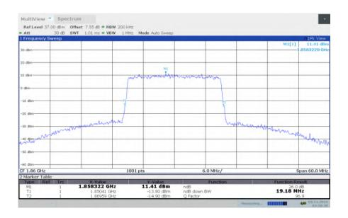
LTE band 2, 20MHz Bandwidth, MID, QPSK (-26dBc BW)
