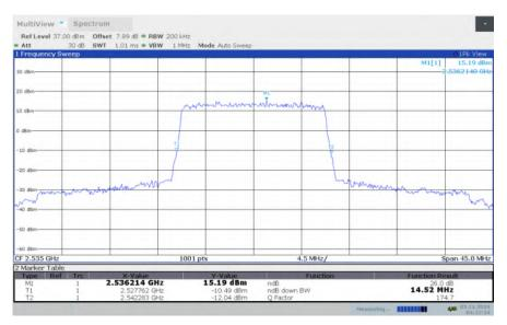
LTE band 7, 15MHz Bandwidth, MID, 16QAM (-26dBc BW)
