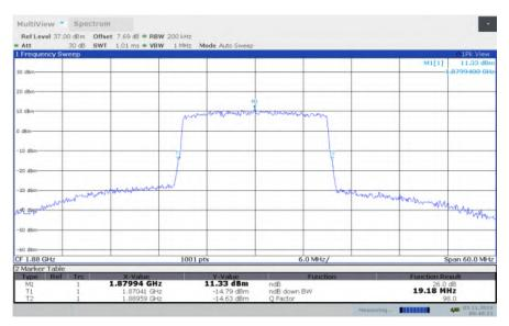
LTE band 2, 20MHz Bandwidth, HIGH, QPSK (-26dBc BW)
