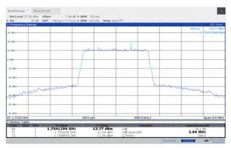
LTE band 4, 3MHz Bandwidth, HIGH, 64QAM (-26dBc BW)
