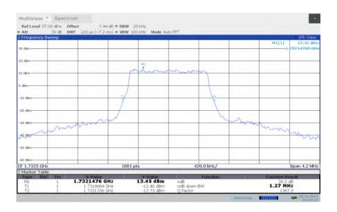
LTE band 4, 1.4MHz Bandwidth, MID, 64QAM (-26dBc BW)
