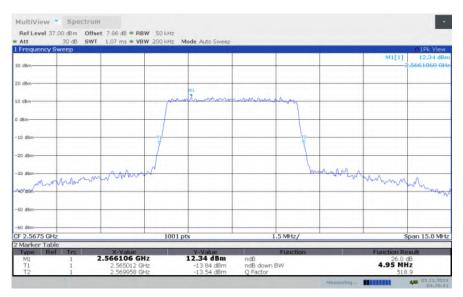
LTE band 7, 5MHz Bandwidth, HIGH, 64QAM (-26dBc BW)
