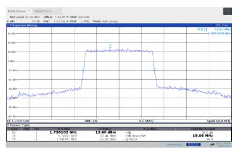
LTE band 4, 20MHz Bandwidth, MID, 16QAM (-26dBc BW)
