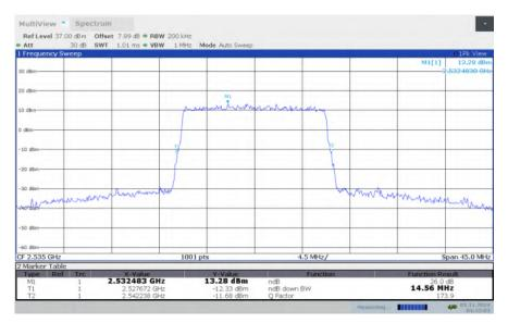
LTE band 7, 15MHz Bandwidth, HIGH, QPSK (-26dBc BW)
