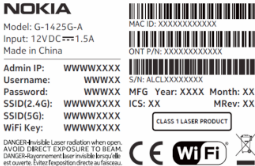
Figure 4-6 Sample laser product safety label on the ONT equipment
