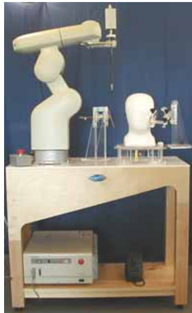
Figure 6: Principal components of the SAR measurement test bench
