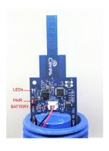
Unscrew the top (cap) to access the sensor controls.
