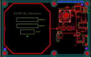
The antenna works on 13.56MHz and the wavelength  $\lambda$  is about 22m (rounded down). The circumference of the antenna is 2x (W+H)=0.24m (rounded up) and the "antenna size" is about 0.011 or  $\lambda$ /90. The inductive coil is small and this is an indication that very little power is radiated and almost all energy is stored as inductive energy in the near field.
