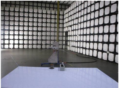
Radiated Emissions (9kHz-30MHz)
