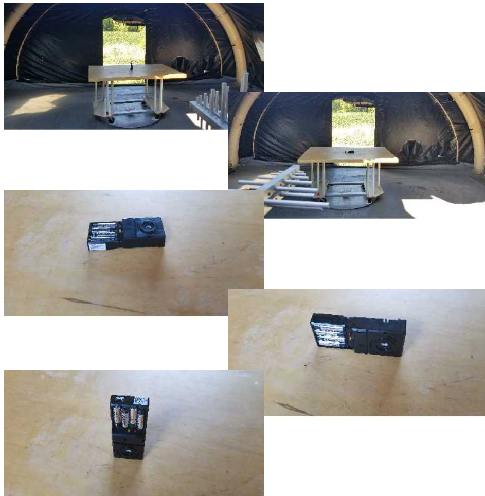
Figure 4: Radiated Emissions Test Setup Photograph(s).
