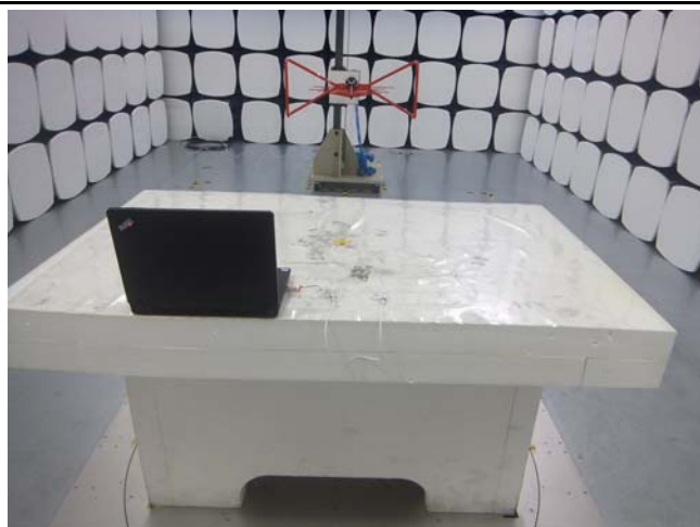
Radiated Spurious Emissions Test Setup Below 1GHz
