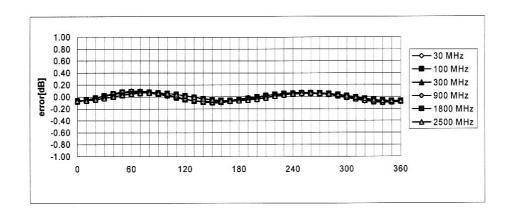
Axial Isotropy Error < ± 0.2 dB
