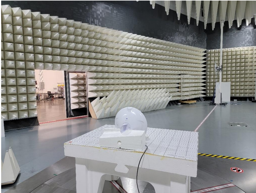
Photograph 1: View Test Set Up Radiated Emissions 30 – 1000 MHz
