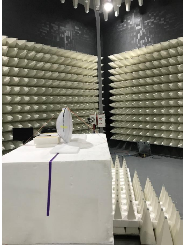
Photograph 3: View Test Set Up Radiated Emissions 17 – 40 GHz
