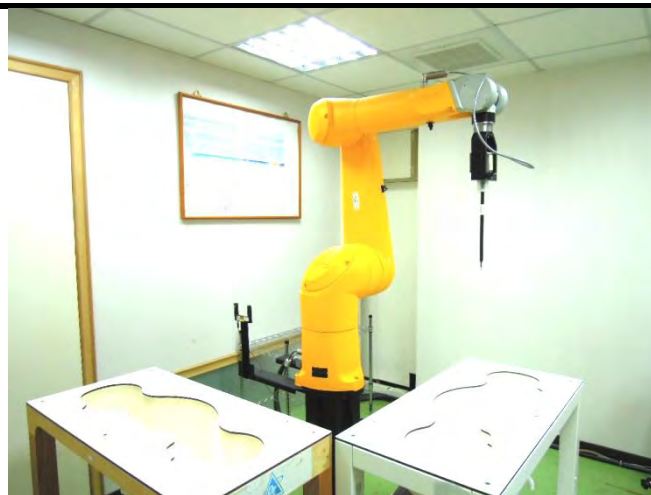
Fig-3.2 SPEAG DASY52 System
