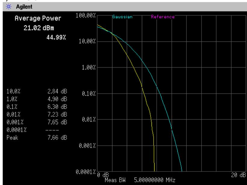
**16QAM, BW 5MHz, RB25-0**
