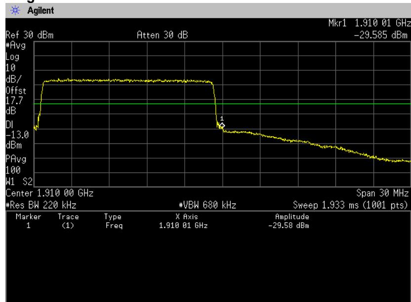
**QPSK, BW 20MHz, RB1-0****Channel: Low**
