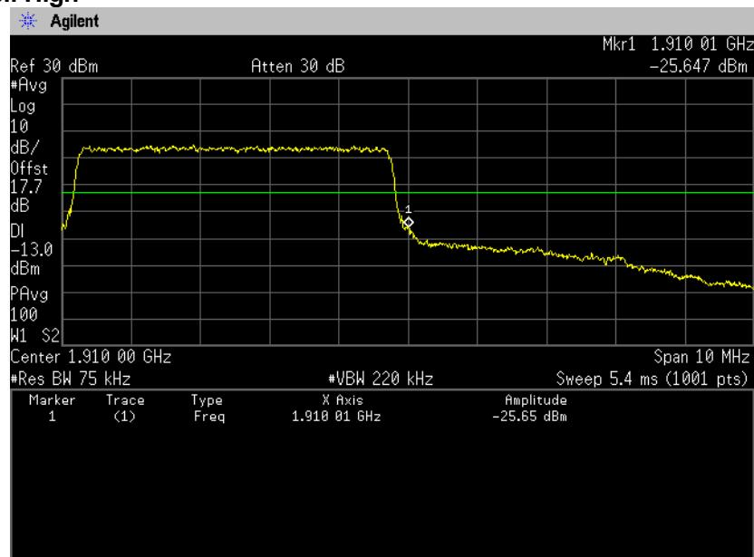
**QPSK, BW 10MHz, RB1-0****Channel: Low**
