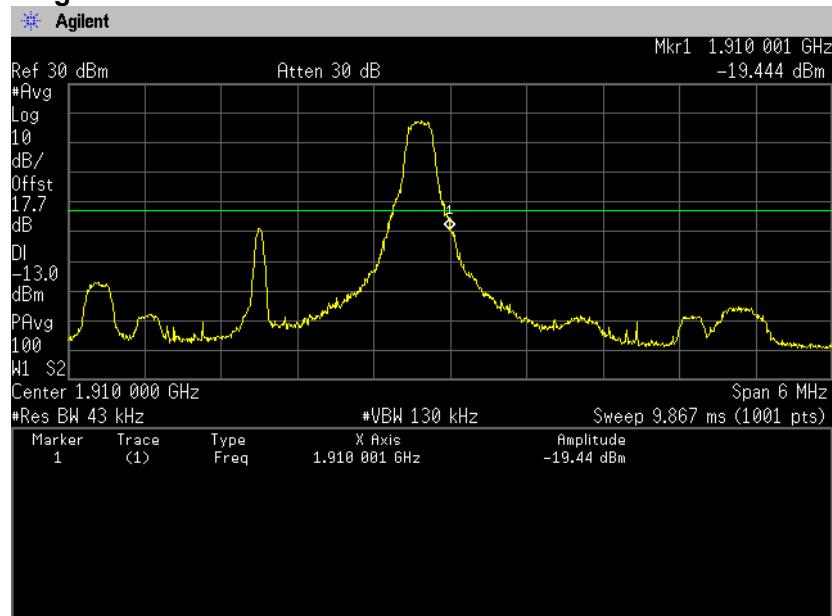
**QPSK, BW 3MHz, RB15-0****Channel: Low**
