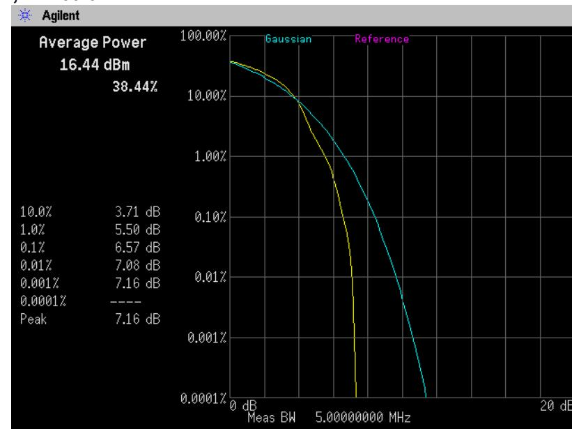
**16QAM, BW 1.4MHz, RB6-0**
