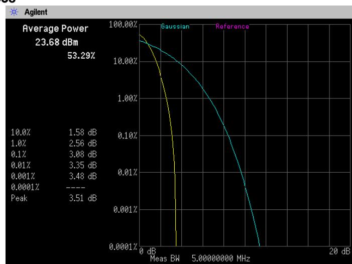
**[LTE Band II]****Channel: 18900****QPSK, BW 1.4MHz, RB6-0**
