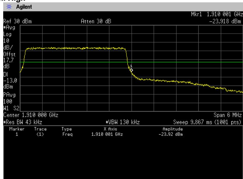
**QPSK, BW 5MHz, RB1-0****Channel: Low**
