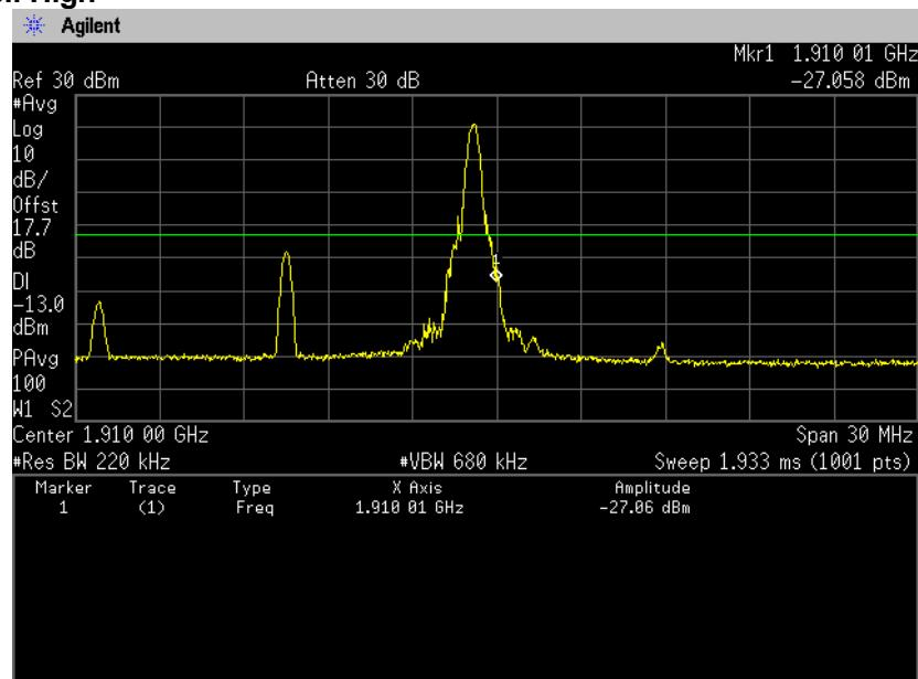
**16QAM, BW 15MHz, RB75-0****Channel: Low**
