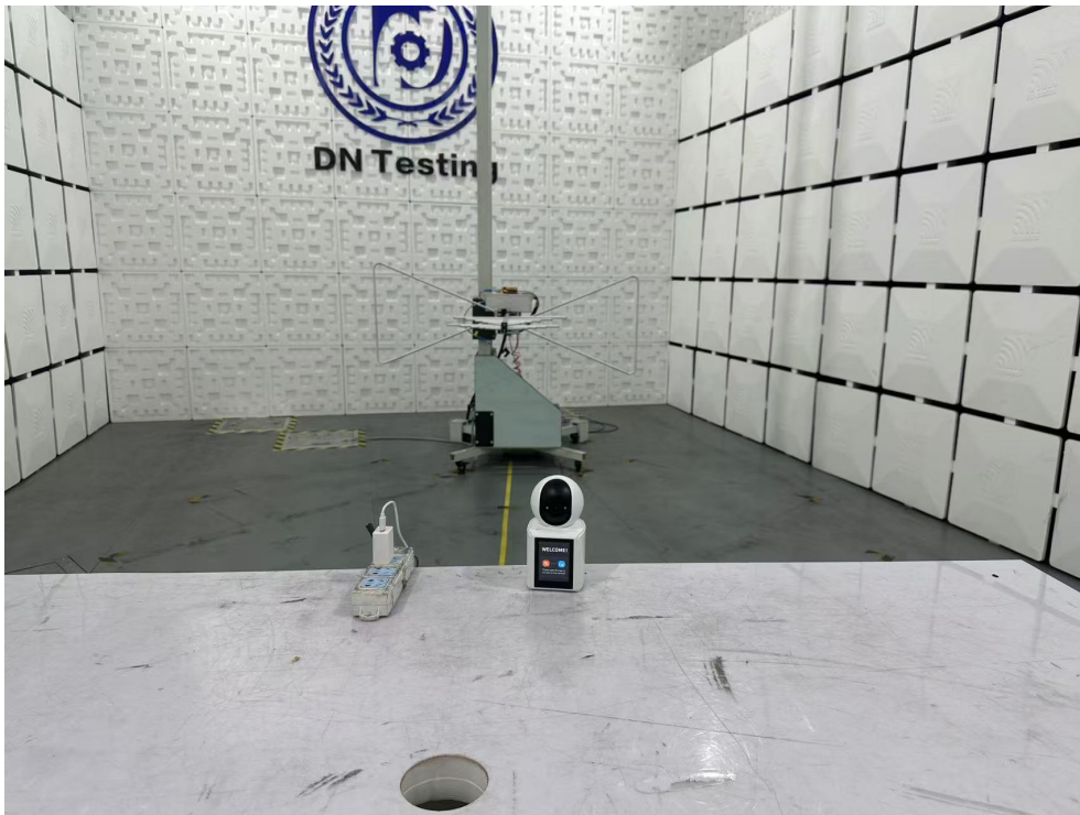
Radiated Emission Test View|(Below 1G)
