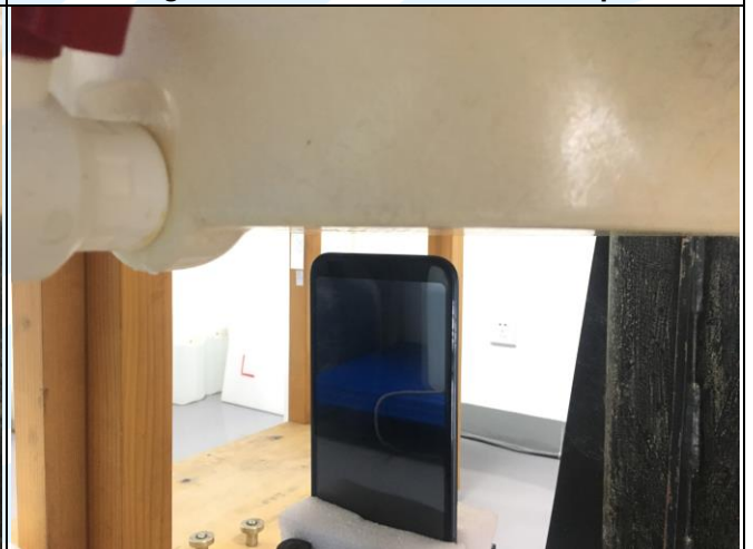
Bottom Side of EUT with 1.0 cm Gap
