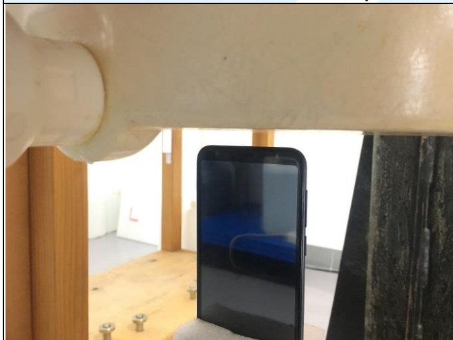
Top Side of EUT with 1.0 cm Gap
