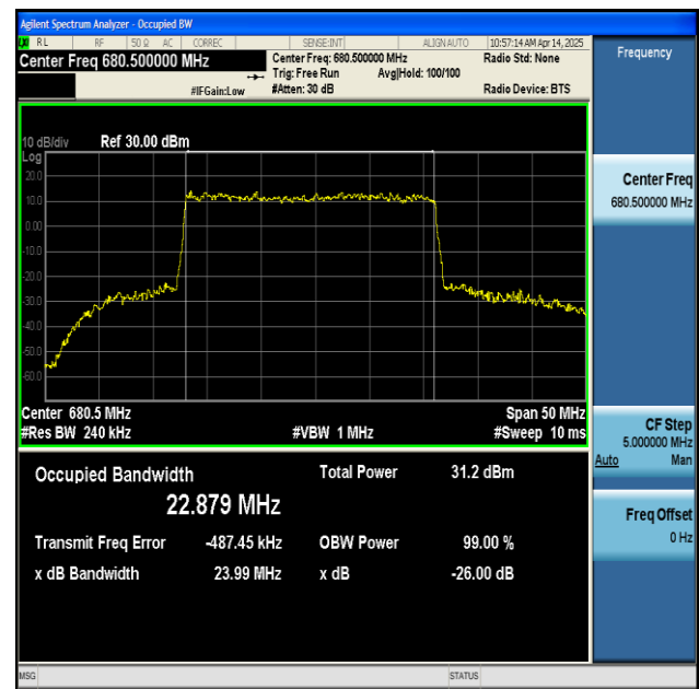
NTNV-n71-PC3-15-25-M-DFT-16QAM-Outer_Full-Ant1-PASS
