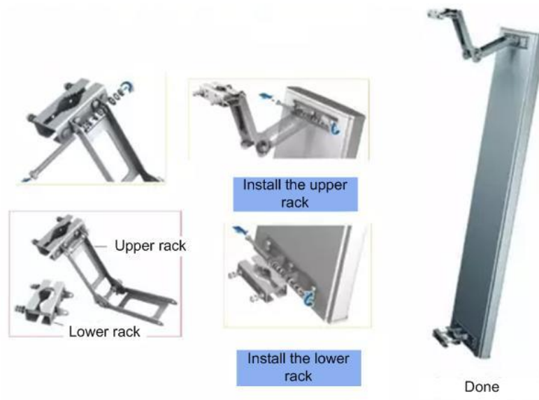
Figure 3-6 Assembling Procedure of Directional Antennas
