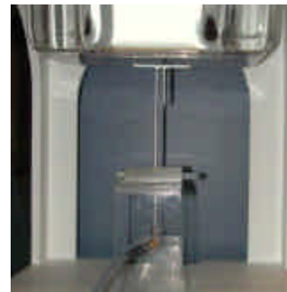
Figure A-1 Dipole Validation Test Setup
