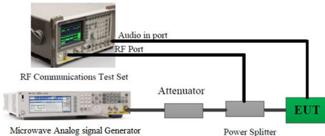
2. Apply a signal to the EUT antenna port at lowest, middle, highest channel frequencies of the operating band;
