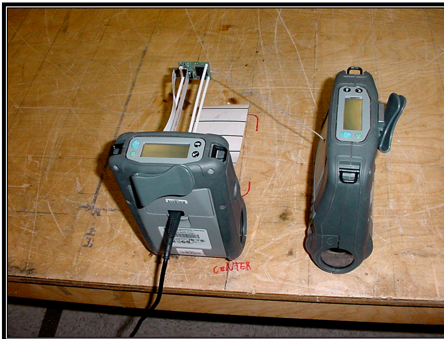
PHOTOGRAPH 12: CONDUCTED EMISSIONS REAR VIEW USING QL-420 CQ17383-1 ANTENNA
