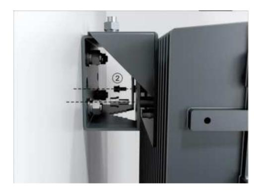
8. Connect and lock the power cable at the H2RU rear side.
