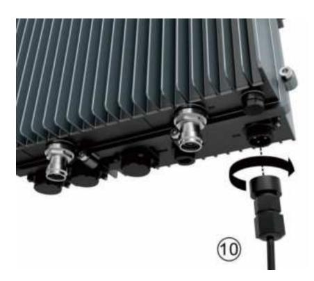
9. Connect and screw the ground cable at the H2RU left side.
