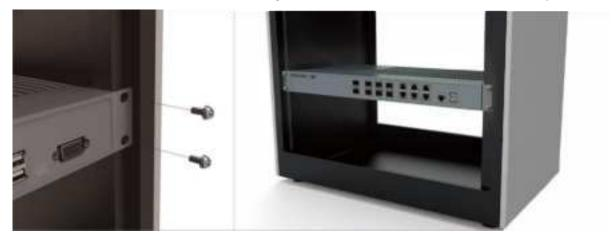
4. Reserve enough free space or Install the fan for cooling if multiple devices are installed in the same rack.
