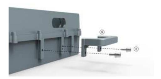
2. Attach and fasten the Bracket I to the back of H2RU with screws M6×14 using T5 Wrench.
