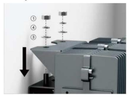
7. Fasten the Bracket I and II with screws M6×14.
