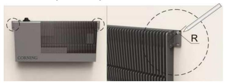
3. Drill 4 holes at the marked sites using percussion drill and embed  $4\times \emptyset 10$  plastic expansion pipes. Note: H = 70 mm. Fasten the case with  $4\times M6$  expansion bolt.
