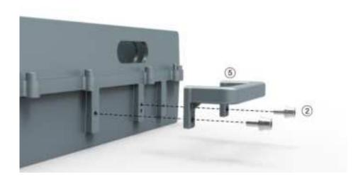
2. Attach and fasten the Bracket I to the left side of H2RU with screws M6×14 using T5 Wrench.
