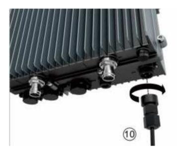
9. Connect and screw the ground cable at the H2RU's left side.
