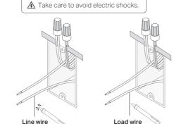
2) Turn off the circuit breaker. Label the Line and Load wires.
