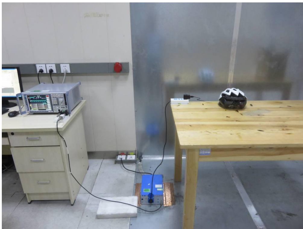
FCC RADIATED EMISSION TEST SETUP
