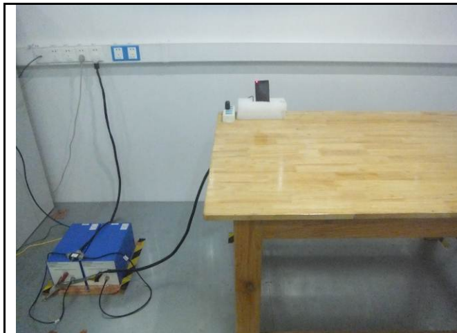
Conducted Emissions Test Setup Front View
