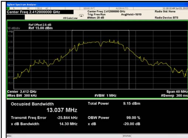
802.11b 20dB Bandwidth - Low CH 2412
