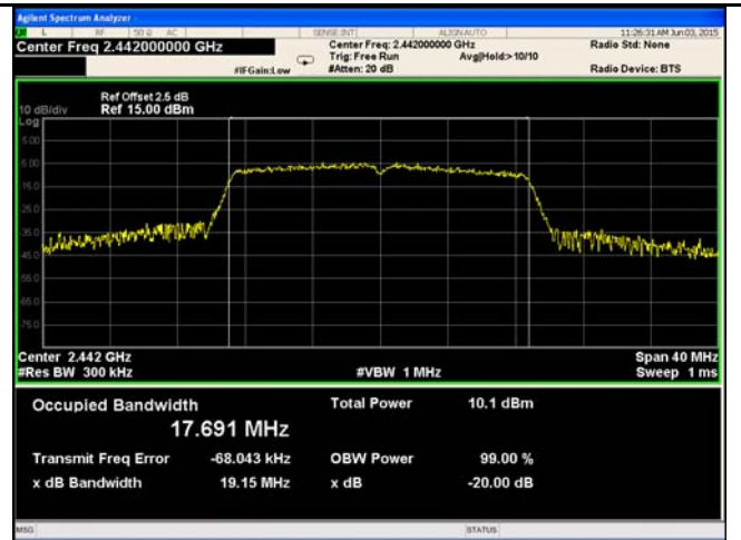
802.11n20 20dB Bandwidth - Mid CH 2442
