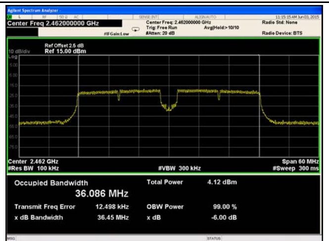
802.11n40 6dB Bandwidth - High CH 2462
