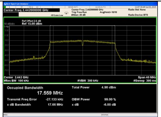
802.11n20 6dB Bandwidth - Mid CH 2442
