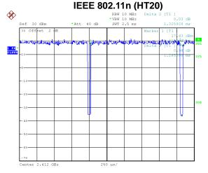
Duty cycle = 2.736 ms / 2.776 ms = 98.56%Duty Factor =  $10 \log(1/\text{Duty cycle}) = 0.00$
