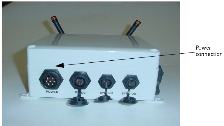
Figure 3-1 Signpost power connection
