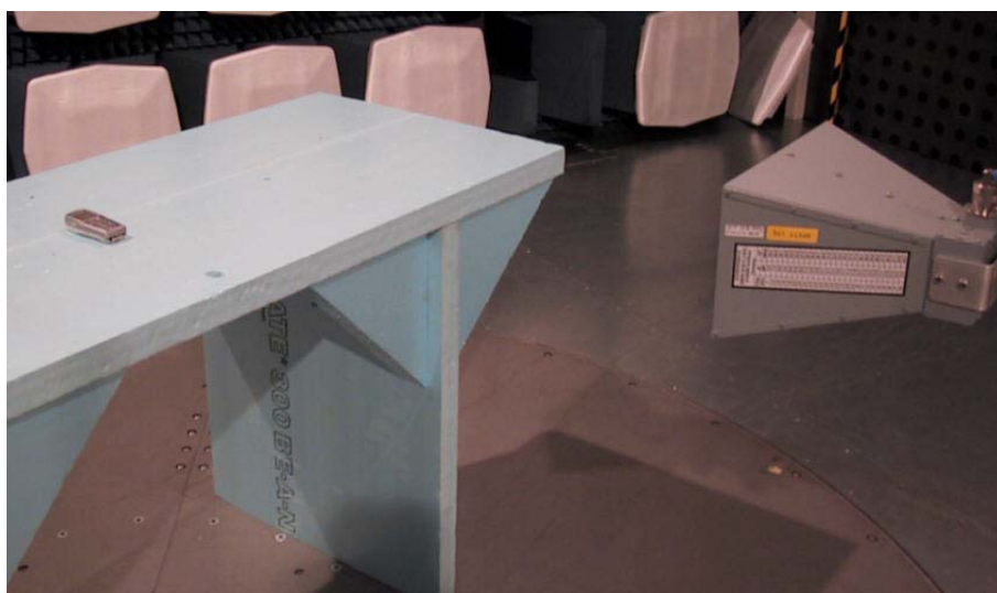
Picture 4: Radiated spurious emission measurement set-up for above 3 GHz measurements, EUT in horizontal orientation
