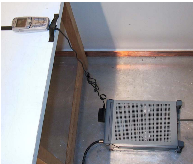
Picture 2: AC-power line conducted emissions test setup
