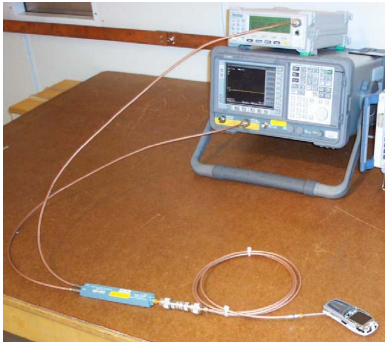
Picture 1: test set-up for conducted measurements from antenna port
