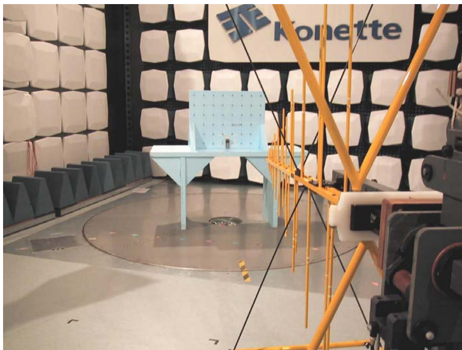
Picture 3: Radiated spurious emission measurement set-up for below 3 GHz measurements, EUT in vertical orientation
