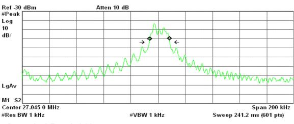
Occupied Bandwidth 14.7992 kHz Occ BW % Pwr 99.00 % x dB -20.00 dB
