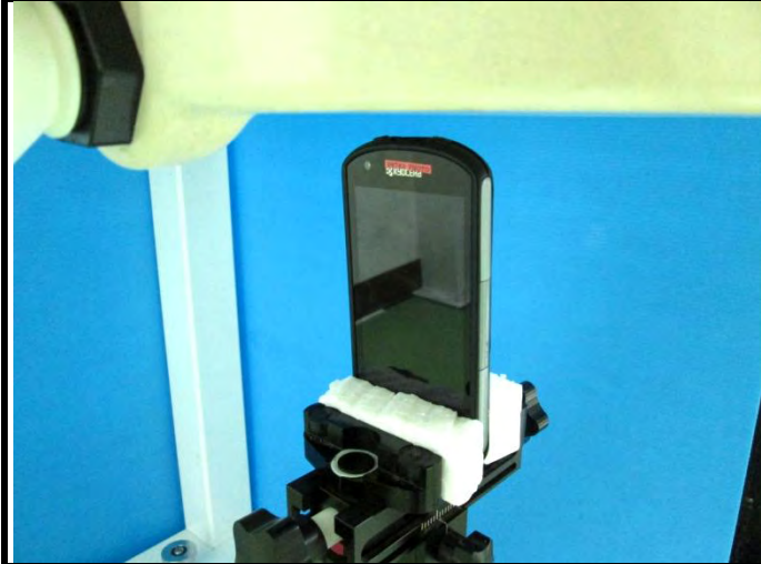
Top Side of EUT with 1.0 cm Gap
