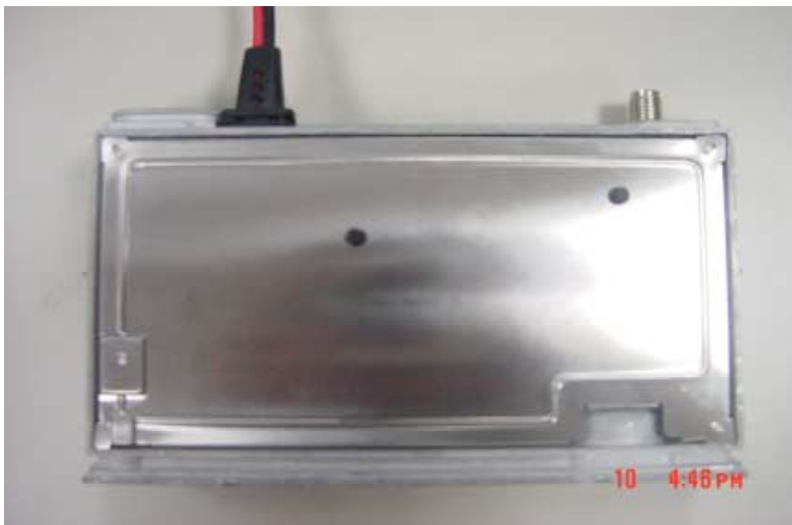
Figure 9-7: Top view of chassis with main shield in place.
