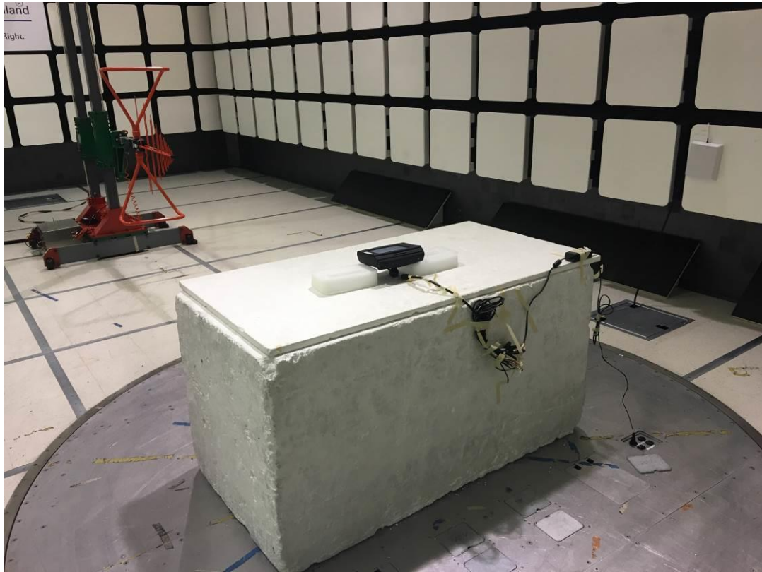
Figure 2: Test Setup for Radiated Emissions 30 MHz to 1000 MHz - Rear
