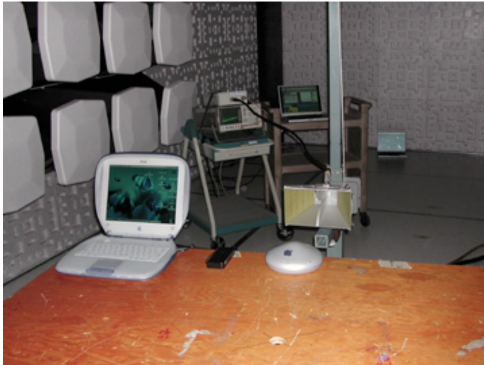
Photo 3 Radiated Emissions Test Setup Above 1 GHz - Front View
