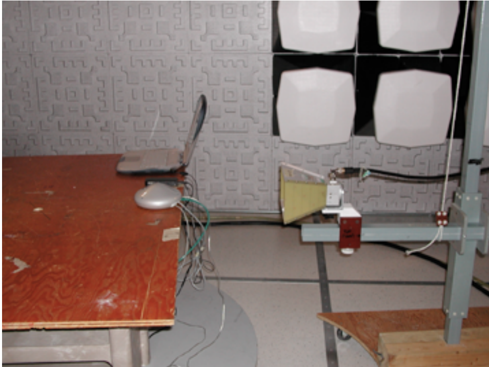
Photo 4 Radiated Emissions Test Setup Above 1 GHz - Side View
