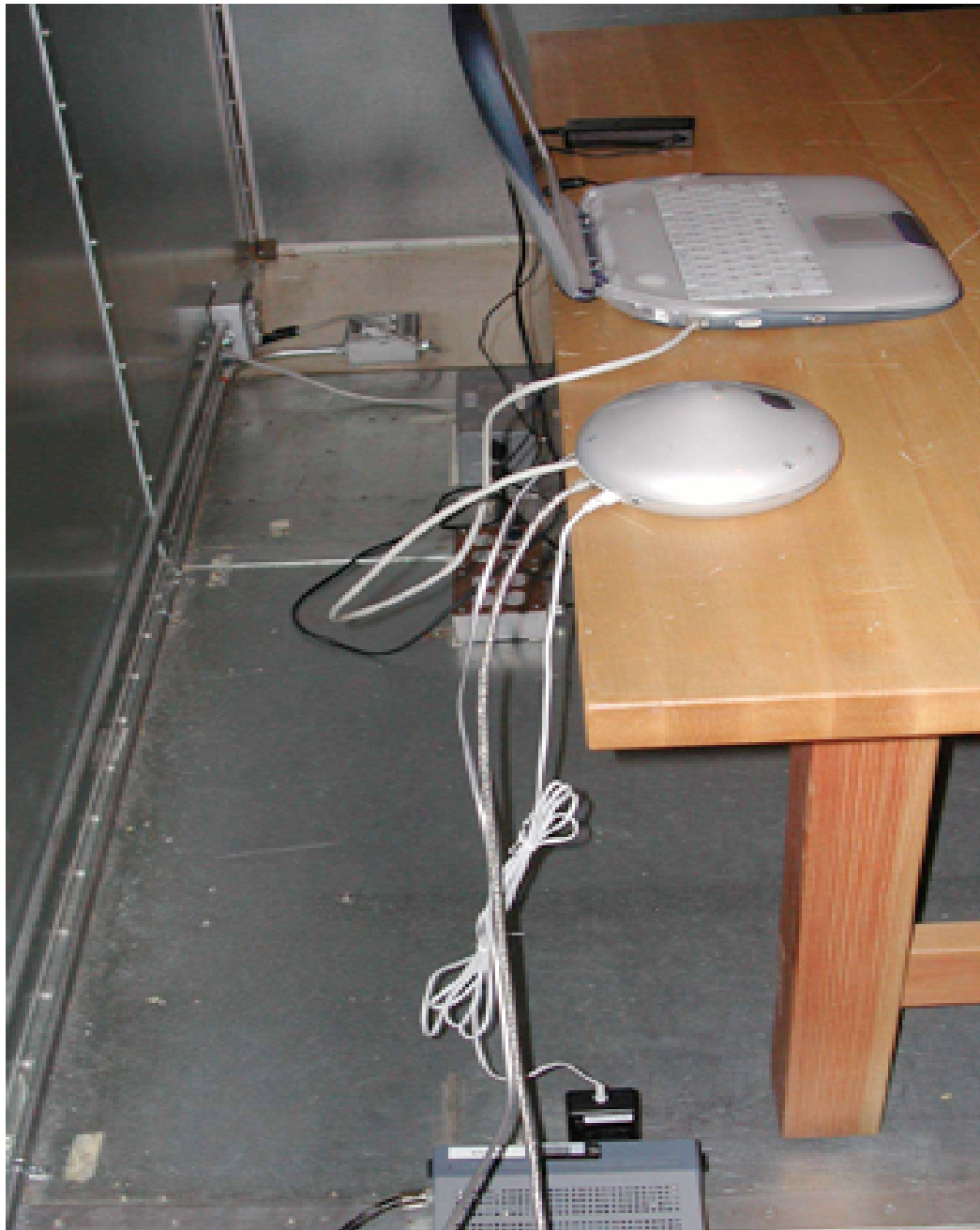
Photo 2 Power Line Conducted Emissions Test Setup - Side View
