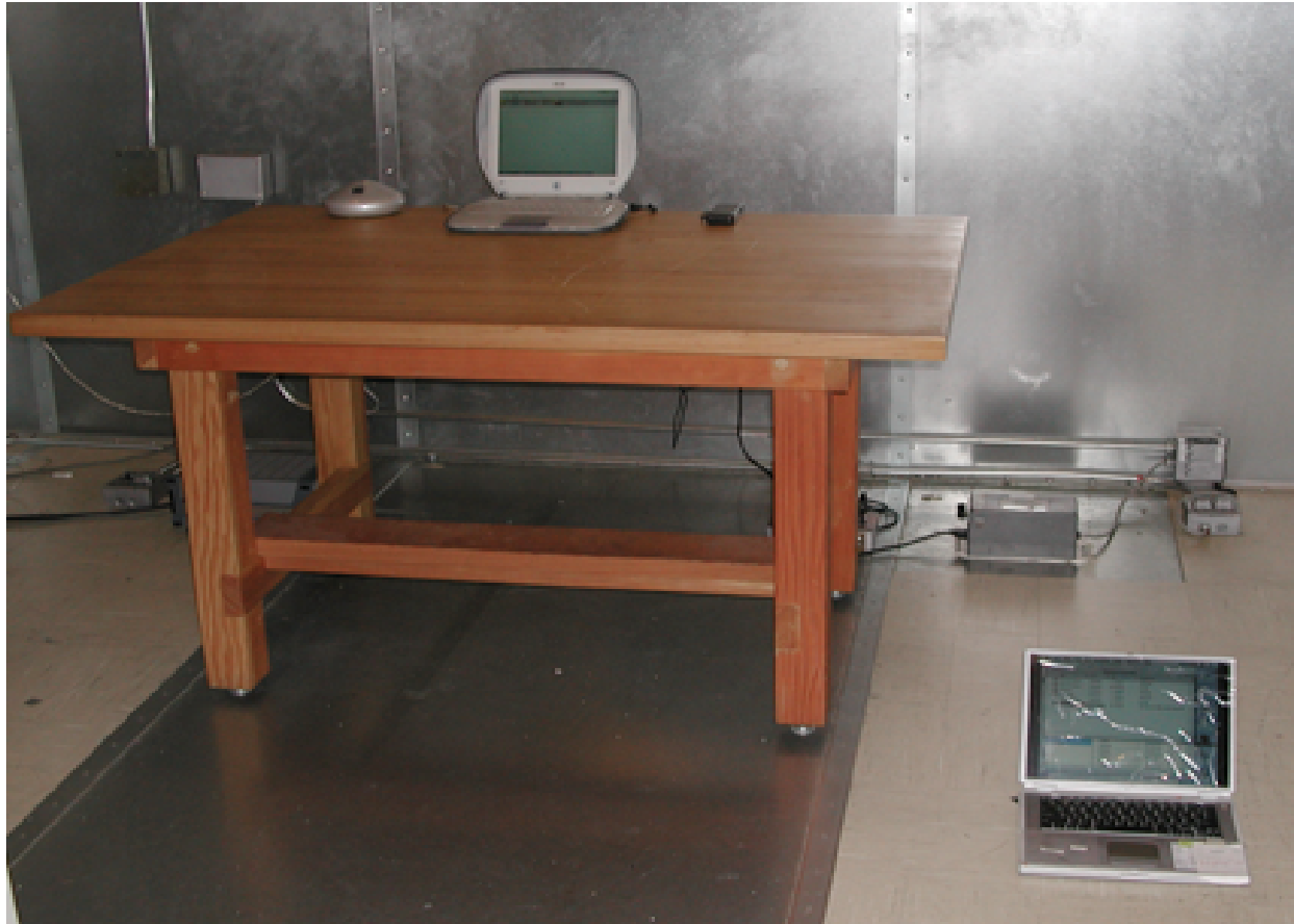
Photo 1 Power Line Conducted Emissions Test Setup - Front View
