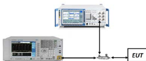
Figure 7-1. Test Instrument & Measurement Setup
