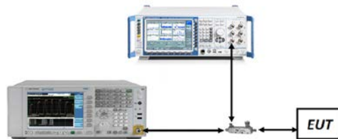
Figure 7-2. Test Instrument & Measurement Setup
