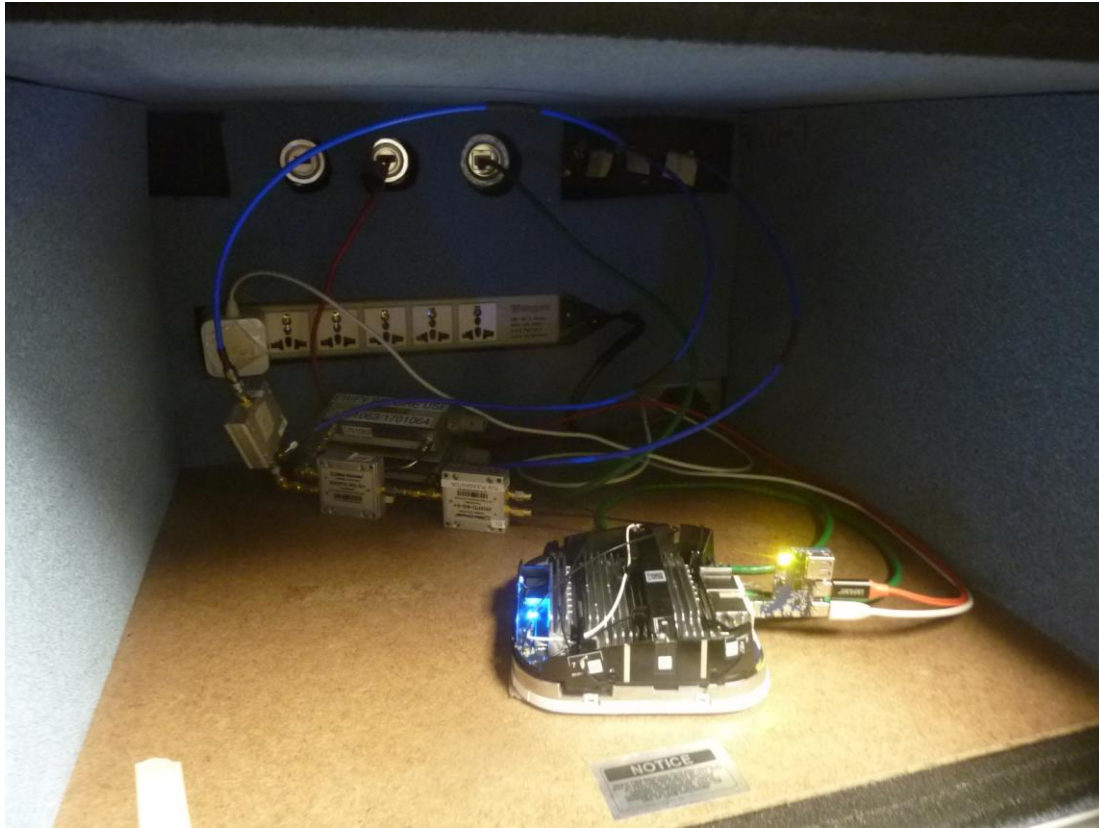
Figure 36: DFS Test Setup Photo for Master – Conducted Method – View 2
