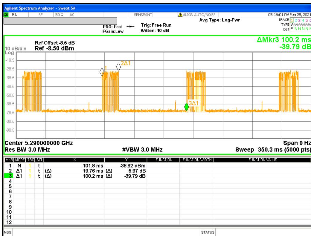
Figure 13: EUT Channel Loading at 5290 MHz (80 MHz bandwidth)
