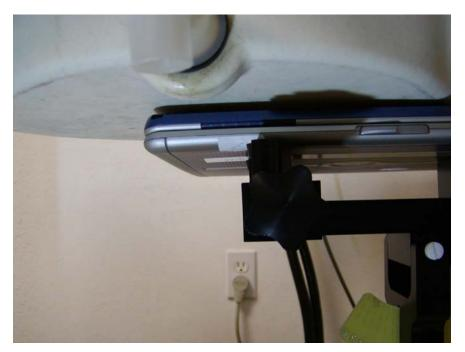
Notebook cover closed perpendicular side touching flat phantom, antenna position left(Aux)(Antenna Model: HFT06)
