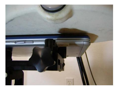
Notebook cover closed bottom side touching flat phantom, antenna position right(main)(Antenna Model:CAO-S)
