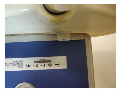
Notebook cover closed perpendicular side touching flat phantom, antenna position right(main)(Antenna Model: HFT06)
