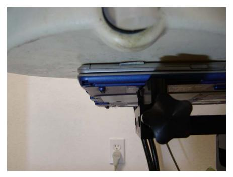
Notebook cover closed top side touching flat phantom, antenna position right(main)(Antenna Model: HFT06)
