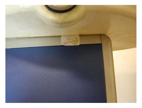
Notebook cover closed perpendicular side touching flat phantom, antenna position right(main).jpg(Antenna Model: CAO-S)  $\,$
