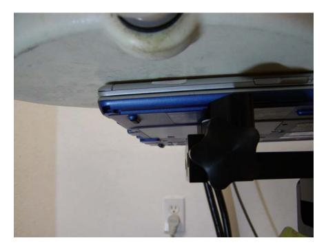
Notebook cover closed top side touching flat phantom, antenna position right(main)(Antenna Model: CAO-S)
