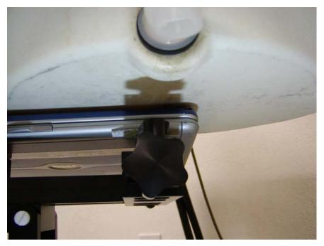
Notebook cover closed bottom side touching flat phantom, antenna position right(main)(Antenna Model: HFT06)
