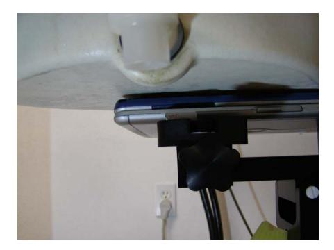
Notebook cover closed perpendicular side touching flat phantom, antenna position left(Aux)(Antenna Model:CAO-S)
