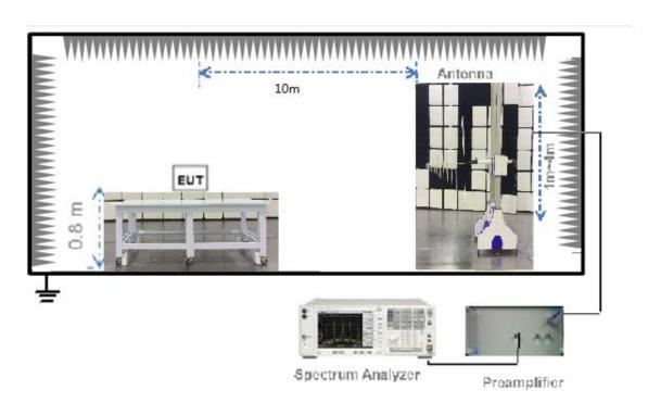
(For Radiated Emission Test (30 MHz-1 GHz))
