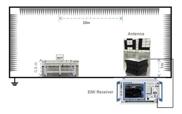
For Radiated Emission Test (Below 30 MHz))
