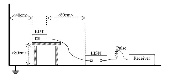
(For Conducted Emission, AC Ports Test)
