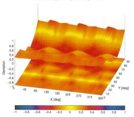
Probe isotropy for  $E_{lot}$ : probe rotated  $\phi=0^\circ$  to 360°, tilted from field propagation direction  $\vec{k}$  Parallel to the field propagation ( $\psi=0^\circ-90^\circ$ ) at 30 GHz: deviation within  $\pm 0.44$  dB Parallel to the field propagation ( $\psi=0^\circ-90^\circ$ ) at 60 GHz: deviation within  $\pm 0.38$  dB
