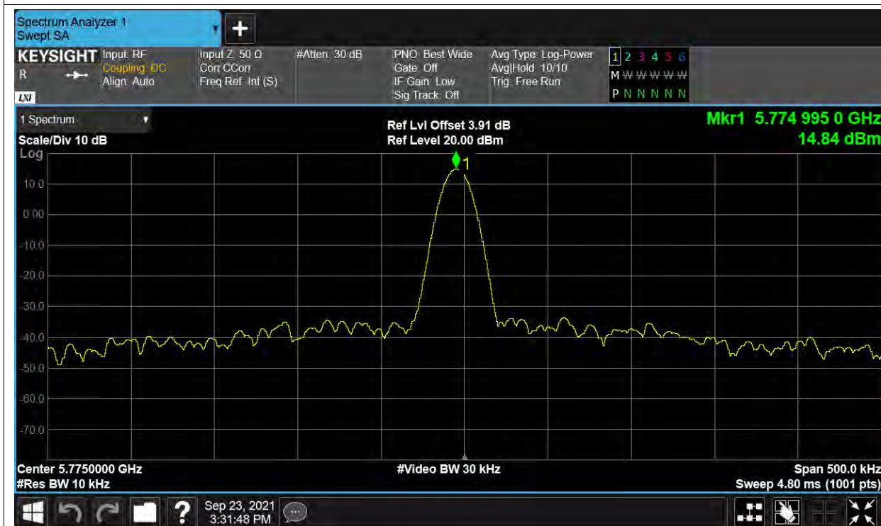
Freq. Stability NVNT ac80 5775MHz MIMO
