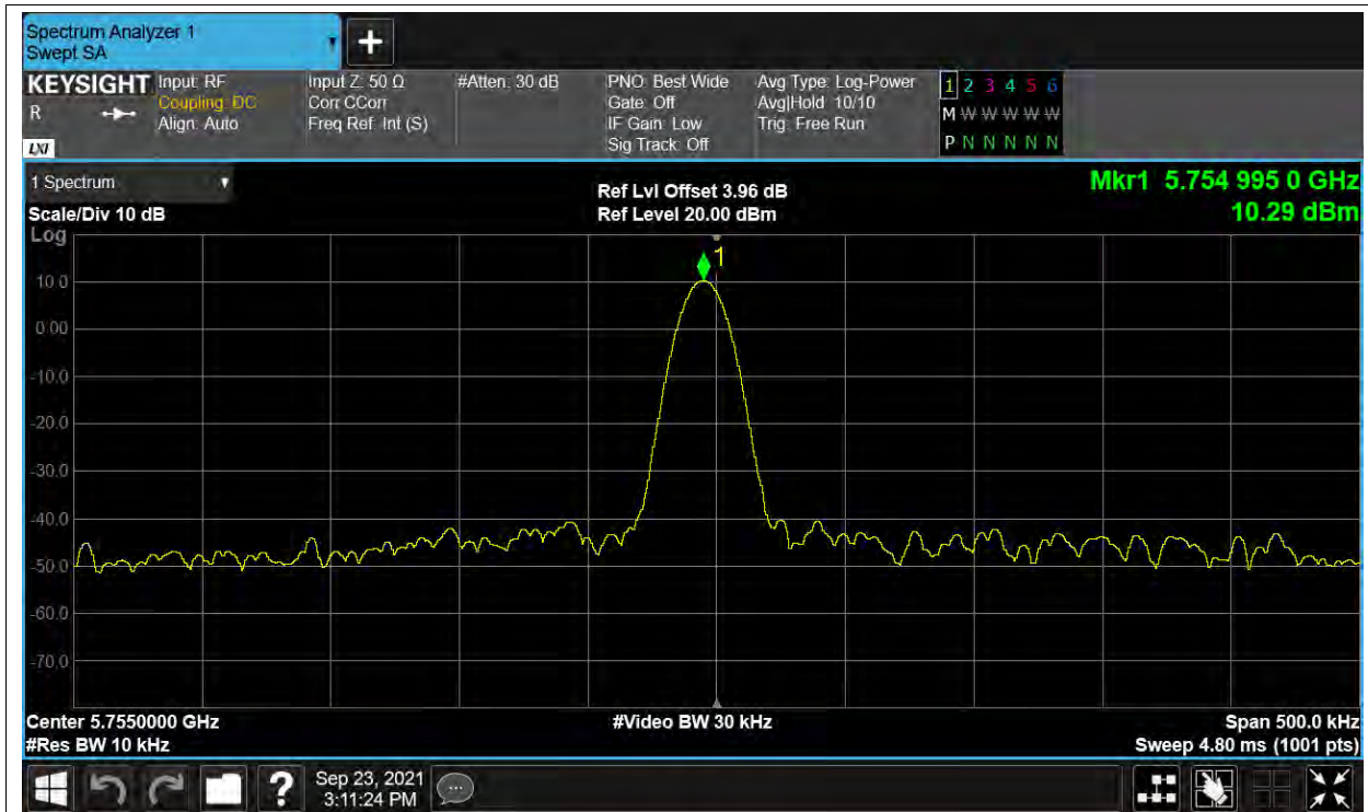
Freq. Stability NVNT ac40 5755MHz MIMO
