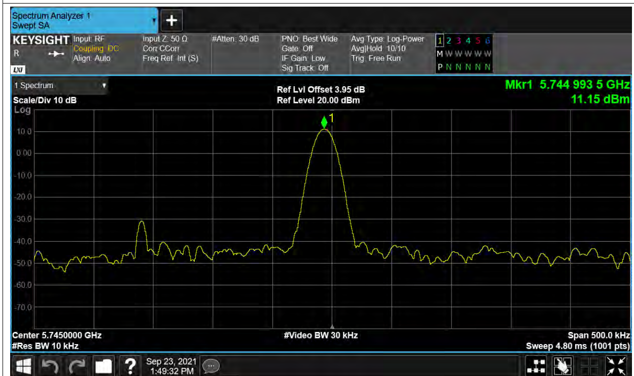
Freq. Stability NVNT n20 5745MHz MIMO
