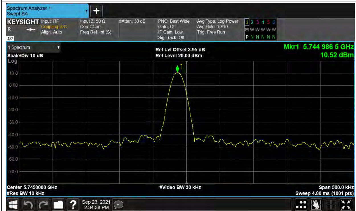
Freq. Stability NVNT ac20 5745MHz MIMO
