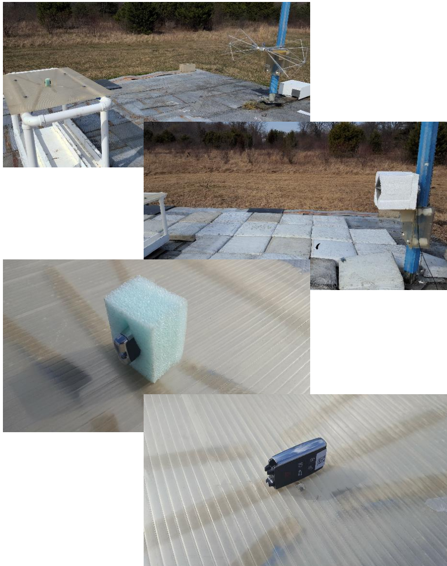
Figure 4: Radiated Emissions Test Setup Photograph(s).
