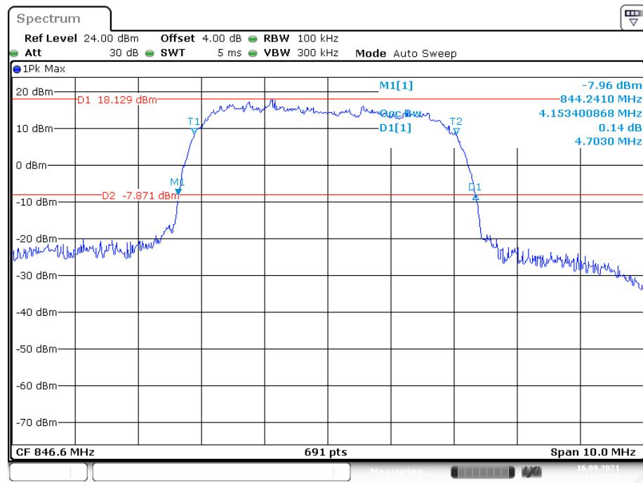
**26 dB Emissions &99% Occupied Bandwidth for HSDPA (16QAM) Mode, Low channel**
