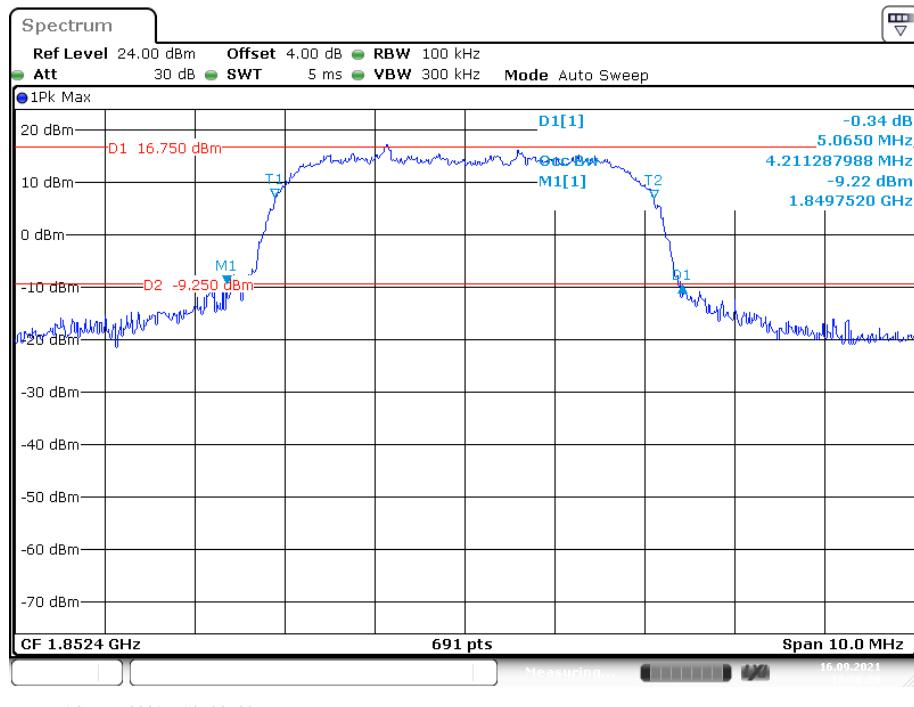
**26 dB Emissions &99% Occupied Bandwidth for HSUPA (BPSK) Mode, Middle channel**
