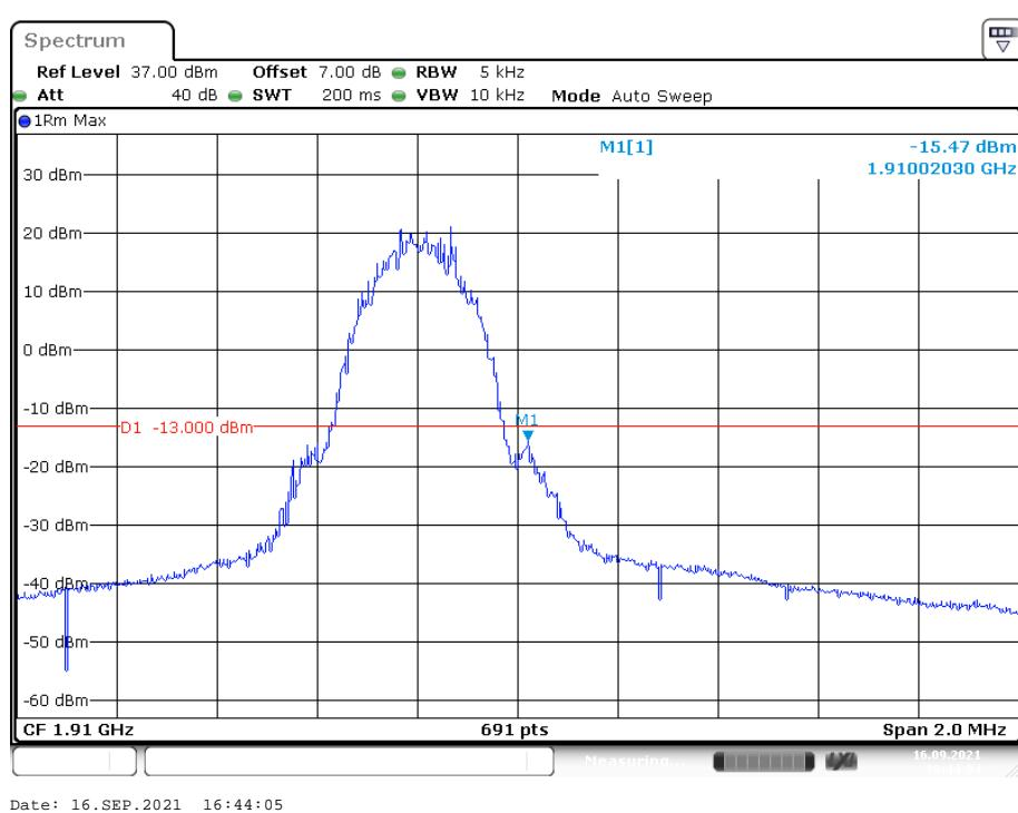
**PCS Band, Left Band Edge for RMC (BPSK) Mode**
