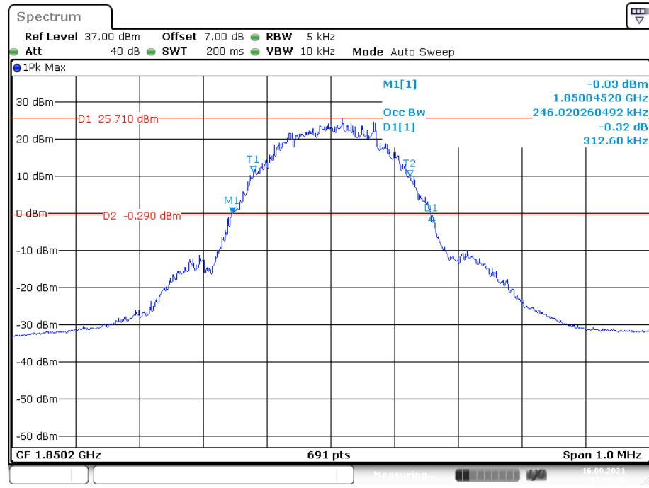
**26 dB Emissions & 99% Occupied Bandwidth for GSM (GMSK) Mode, Middle channel**
