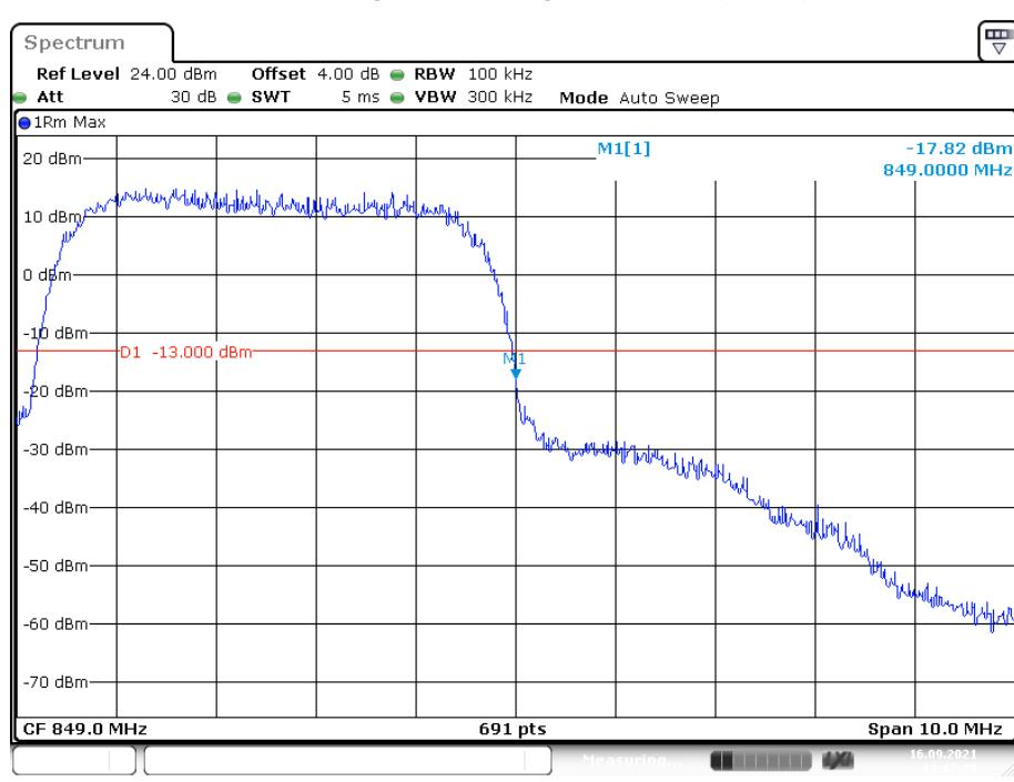
**Cellular Band, Left Band Edge for HSDPA (16QAM) Mode**
