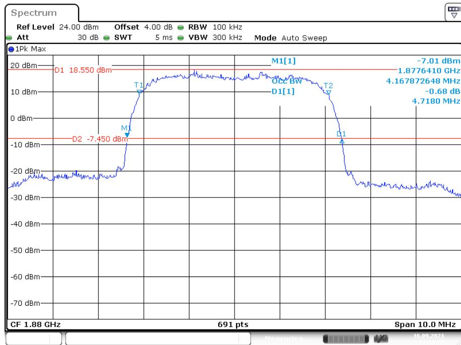
**26 dB Emissions &99% Occupied Bandwidth for RMC (BPSK) Mode, High channel**
