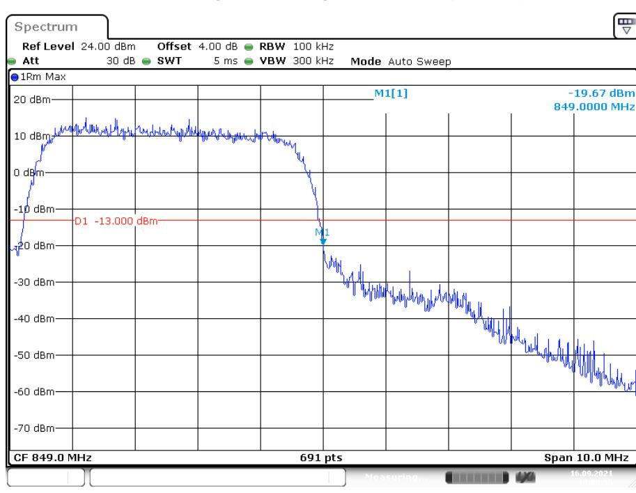
**Cellular Band, Left Band Edge for HSUPA (BPSK) Mode**
