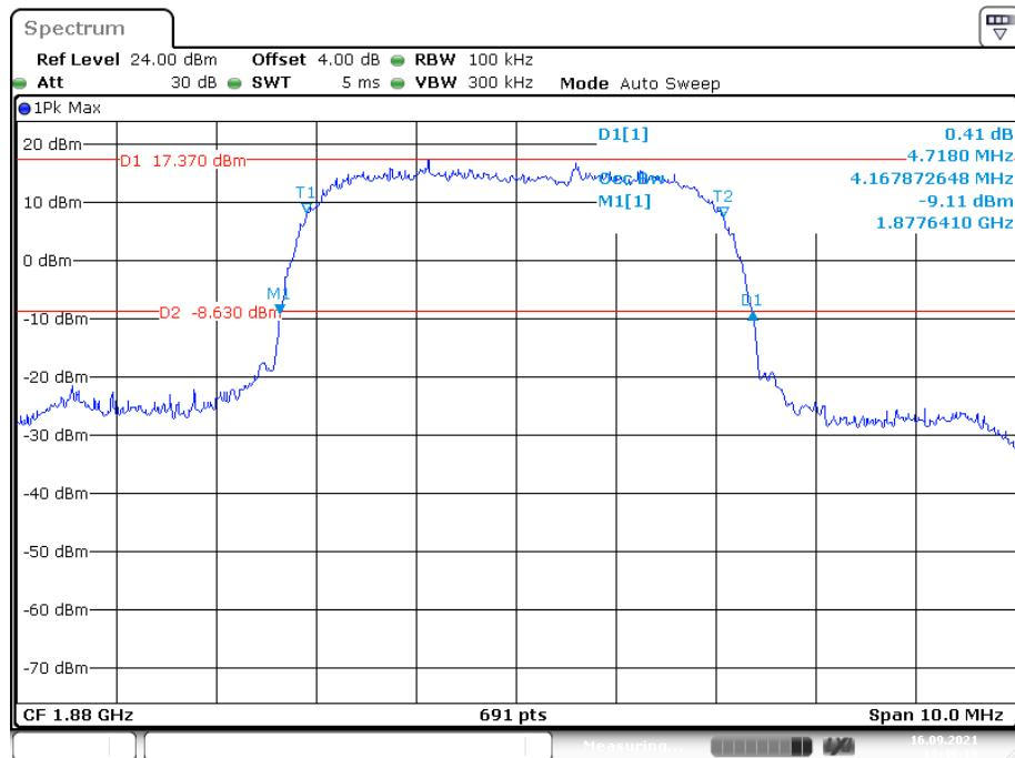
**26 dB Emissions &99% Occupied Bandwidth for HSDPA (16QAM) Mode, High channel**
