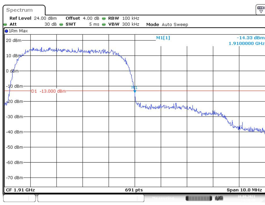
**PCS Band, Left Band Edge for HSDPA (16QAM) Mode**
