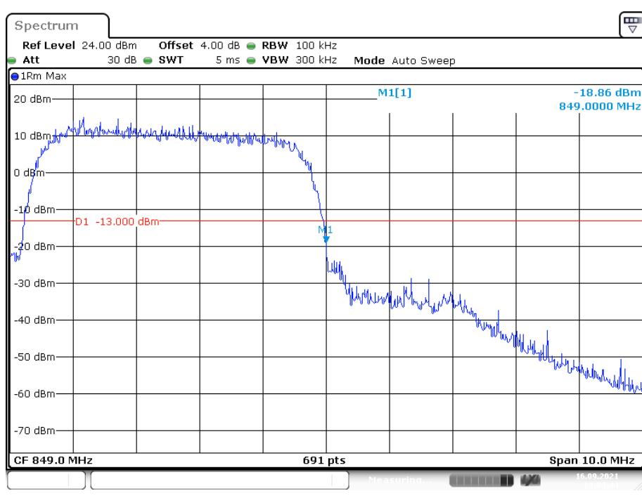
**PCS Band, Left Band Edge for GSM (GMSK) Mode**
