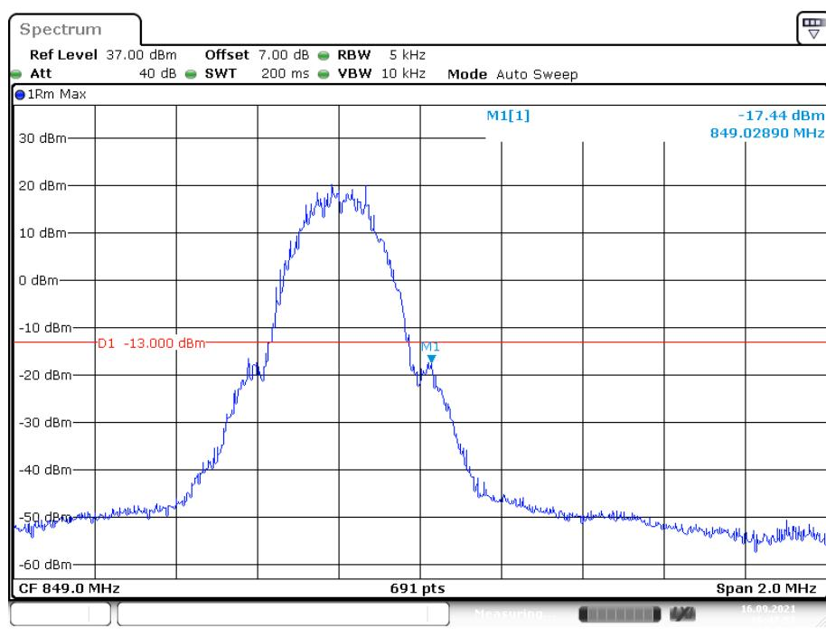
**Cellular Band, Left Band Edge for RMC (BPSK) Mode**
