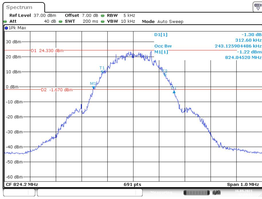
**26 dB Emissions & 99% Occupied Bandwidth for GSM (GMSK) Mode, Middle channel**
