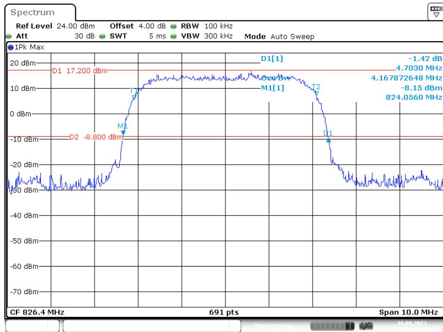
**26 dB Emissions &99% Occupied Bandwidth for HSUPA (BPSK) Mode, Middle channel**
