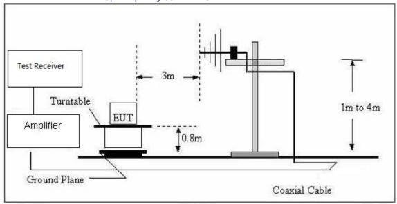
(C) Radiated Emission Test-Up Frequency Above 1GHz
