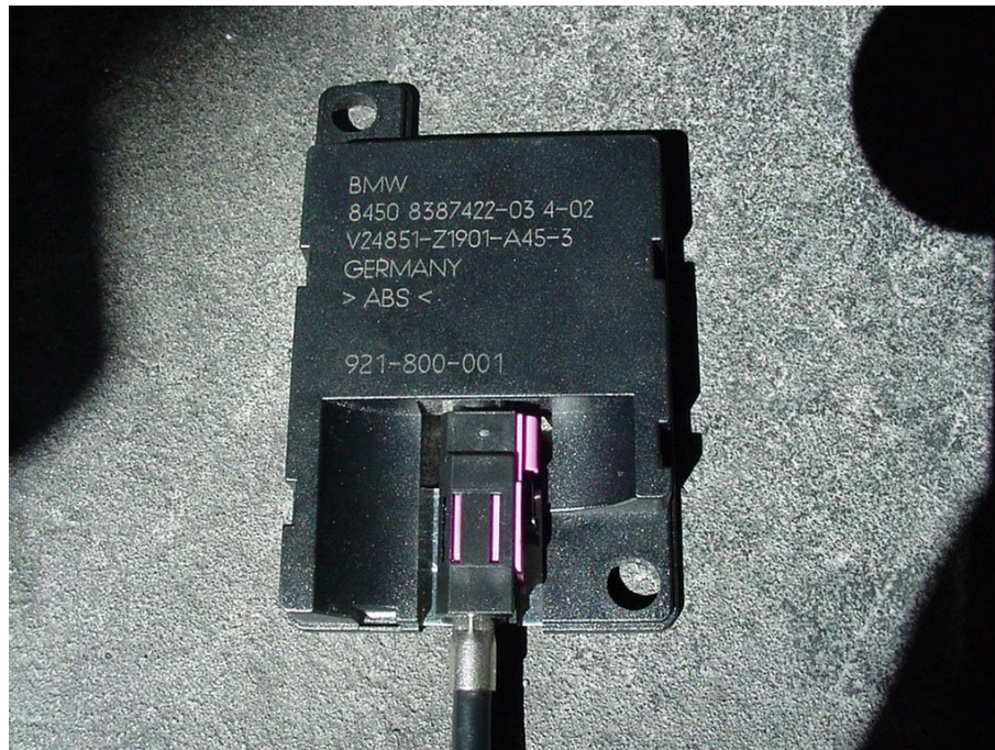
Picture 3 : external antenna
