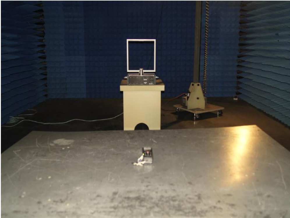
Photograph 2: Set-up for Radiated Spurious Emissions, 30MHz-1GHz
