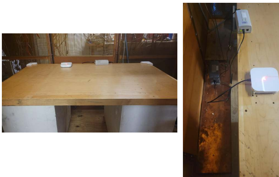
Figure 6: Conducted Emissions Test Setup Photograph(s).
