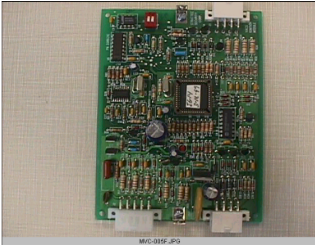
Strattec - PCB up close, Component Side
