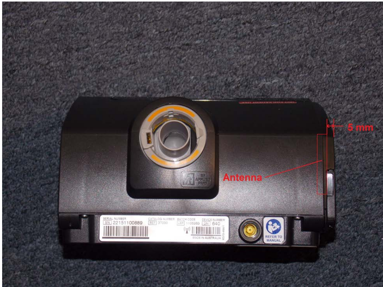
Antenna Location on Back & Distance to End
